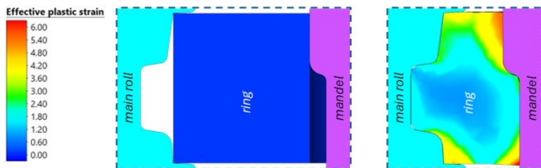
Fig.3 - Comparison distribution in the cross-section of the profiled ring within the radial roll gap before and after the ring rolling process.
