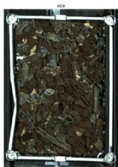
Fig.2 - Stereo camera image for scrap pile height detection: Half full (right) and full (left) scrap box.
