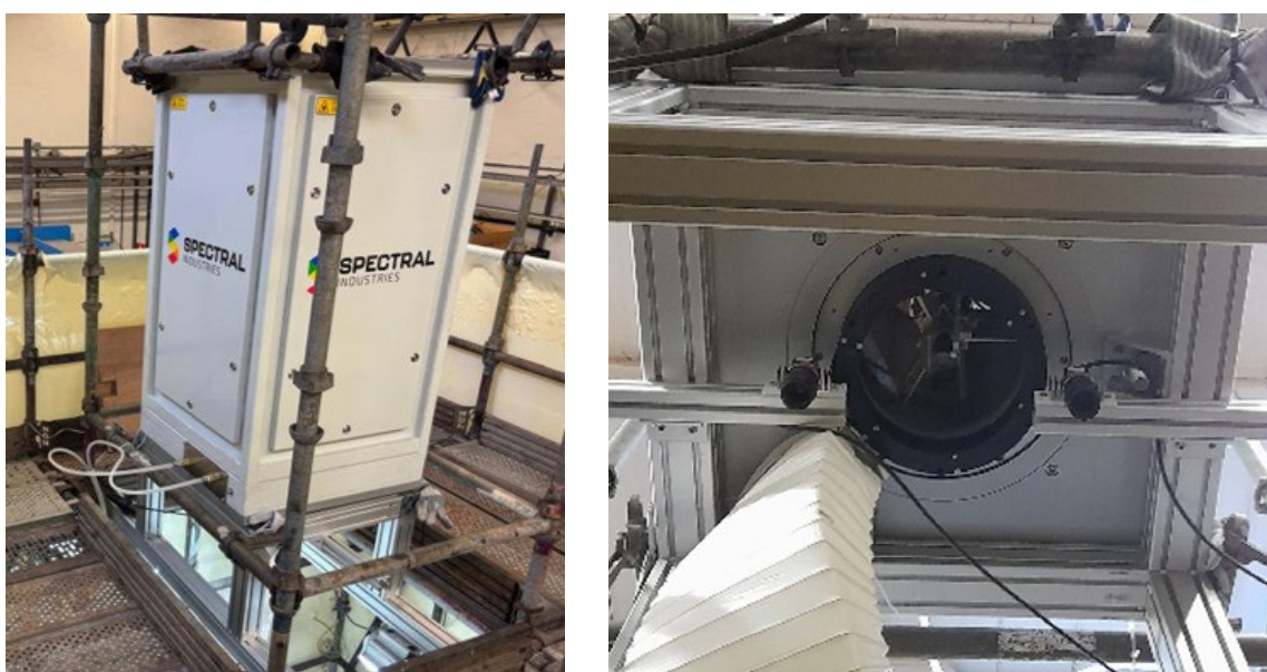
Fig.5 - LIBS analyser mounted on a gantry: Top view (left) and bottom view with stereo camera (right).
