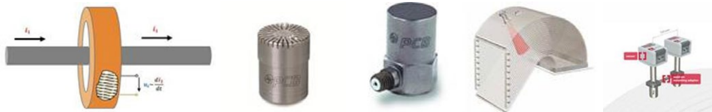
Fig.10 - Components of the multimodal sensor system: Rogowski coils, microphones, vibration sensors and off-gas analysis.
