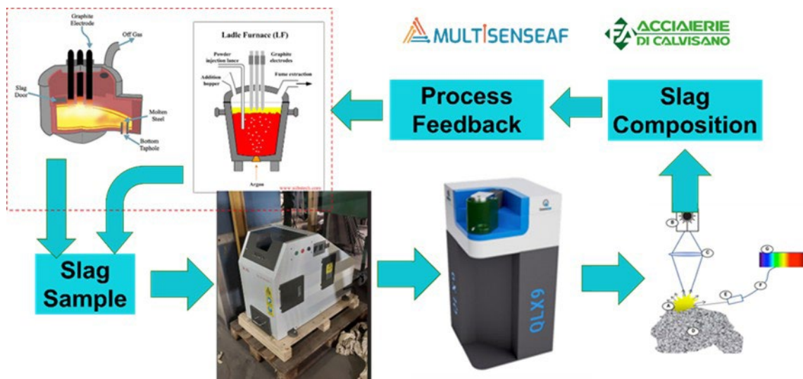
Fig.4 - Control loop of application of fast slag analysis system on the EAF/LF process management.
