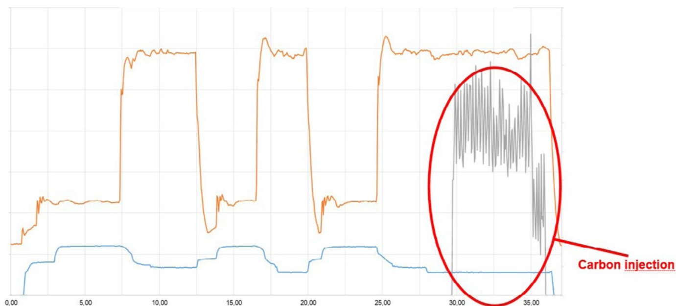
Fig.8 - Graph of consumption values of oxygen (orange line), natural gas (blue line) and injection carbon (black line) as example for a heat during trial period.
