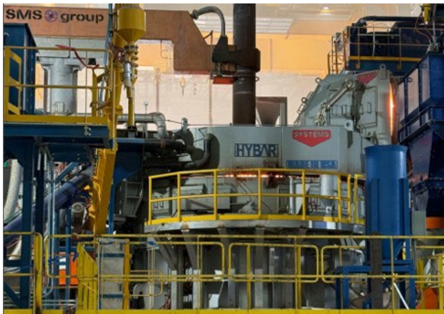
Fig.7 - EAF EDGE design: Spray-Cooled™ upper shell and roof.
