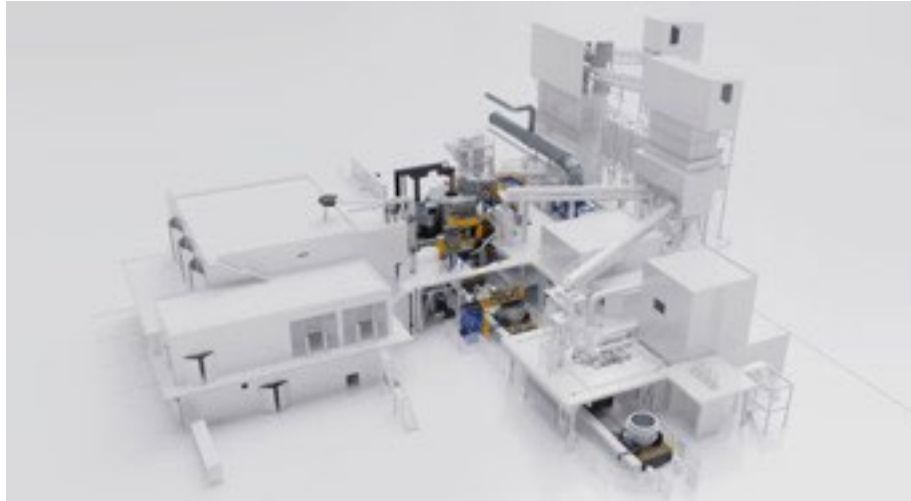
Fig.3 - EAF and LF area layout.
