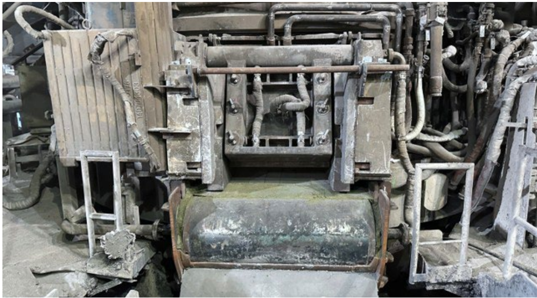
Fig.6 - PTI SwingDoor™ outside view C.M.E.
