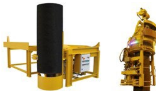
Fig.8 - Electrode handling and jointing [6].
