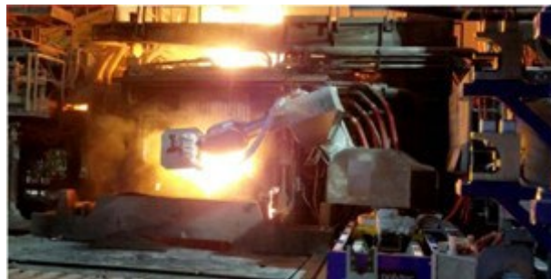
Fig.5 - Fully automated EAF T+P robot (temperature and probe) [4].
