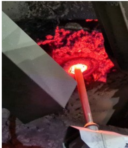
Fig.6 - THM entering taphole for cleaning.
