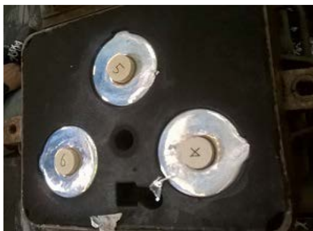
Fig.4 - Test in fonderia. Cilindro N.5 INOLP1 + INOP2; cilindro N.6 INOL1 + INOP2, cilindro X INOX / Foundry test. Cylinder No.5 INOLP1 + INOP2; cylinder No.6 INOL1 + INOP2, cylinder X INOX.
