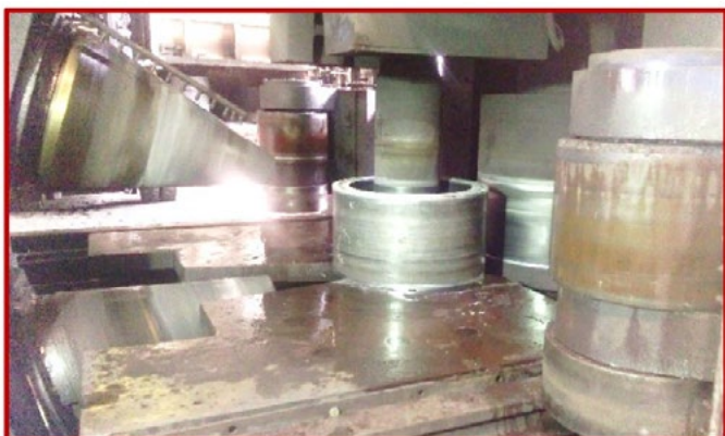
Fig.1 - Cold rolling of ring in rolling mill.
