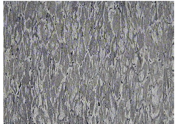
Fig.5 - Grain size ASTM No.4 in Axial Specimens.
