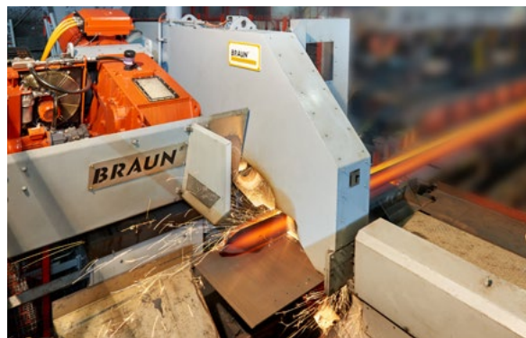
Fig.10 - Abrasive cut-off machine, type TS 16 L, for hot cutting of rails in rail rolling mill, for crop cutting of rails (voestalpine Rail Technology, Donawitz, Austria).
