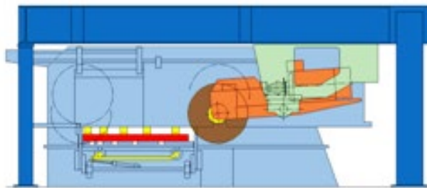
Fig.13 - Principle of BRAUN gantry-type traverse abrasive cut-off machine, type FP.
