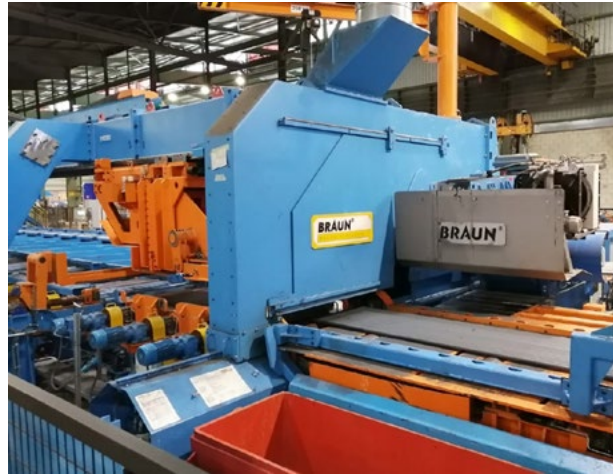
Fig.12 - Traverse cut-off machine, type TS 16 F for warm cutting of bars in layers (SIDENOR Basauri, Spain).
