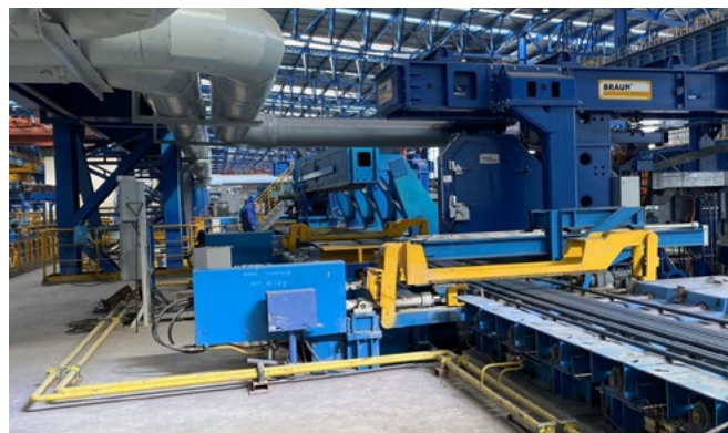
Fig.14 - Gantry-type traverse abrasive cut-off machines, type TS 12 FP, for warm cutting of up to 1600 mm wide layers of bars (SHIGANG, Shijiazhuang, China).
