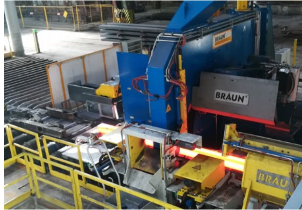
Fig.8 - Abrasive cut-off machine, type TS 16 W, for hot cutting of heavy bars (Acciaierie Valbruna Bolzano, Italy)
