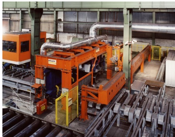
Fig.15 - Gantry-type traverse abrasive cut-off machine, type TS 12 FP, for hot cutting of plates and sheets as well as cold cutting of slabs (BÖHLER Bleche, Austria).
