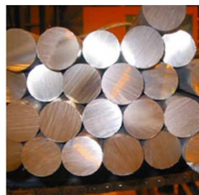
Fig.3 - abrasive cut bar ends.
