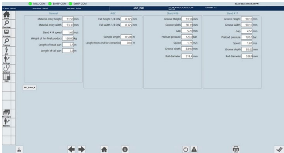
Fig.16 - HMI parameter setting for AGC.
