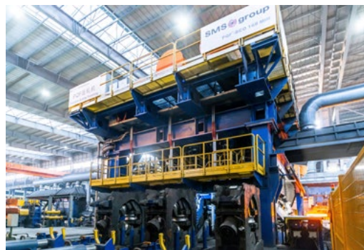
Fig.1 - Advanced third PQF® generation with six rolling stands.
