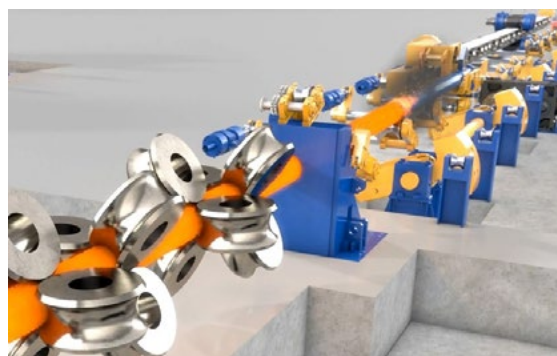
Fig.4 - PQF® rolling process with fast inlet side for rapid mandrel handling.
