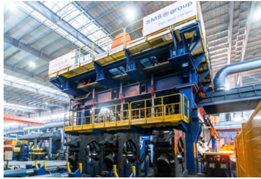
Fig.7 - Side view with PQF® rolling stands for change-over operation.
