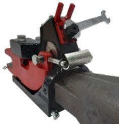
Fig.3 - Single-point adjustment to manually set the gap.
