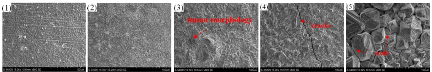
Fig.5 - Oxide film morphology under different temperature (1:900°C, 2:950°C, 3:1050°C, 4:1100°C, 5:1150°C).
