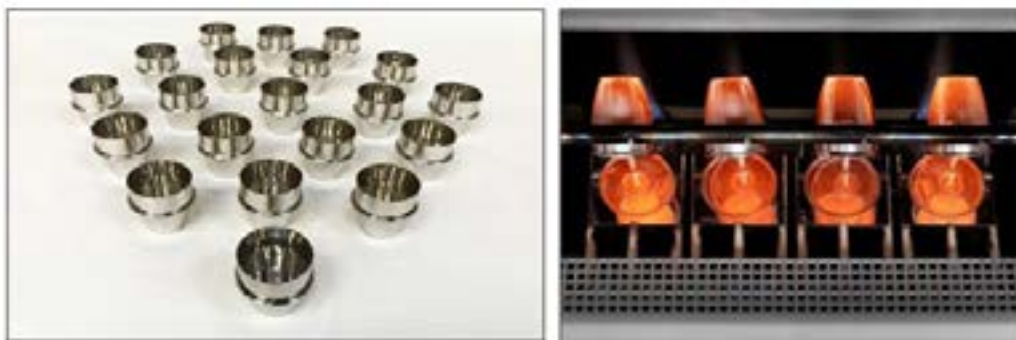
Fig.5 - A sinistra: crogioli da laboratorio in lega platino-iridio. A destra: crogioli e piattini in lega platino-oro 95-5 per perlatrice automatica. Diffusione foto acconsentita da CIMI S.p.A. [15] / Left: platinum-iridium laboratory crucibles. Right: platinum-gold 95-5 crucibles and plates for automatic fusion machine. The photos publication is authorized by CIMI S.p.A. [15].
