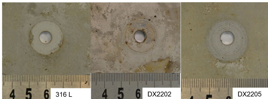
Fig.7 - Typical aspect of corroded samples after 1-year immersion in the pretreatment unit of the Cap Sicié plant.
