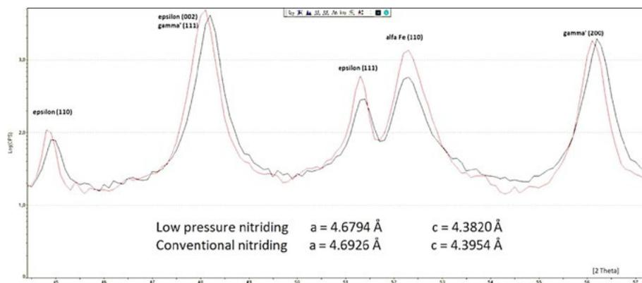
Fig.8 -X-ray diffraction spectra of low-pressure (----- black line) and conventionally (----- red line) nitrided samples. Below the background, the derived cell parameters of the  $\epsilon$ -phases are reported.
