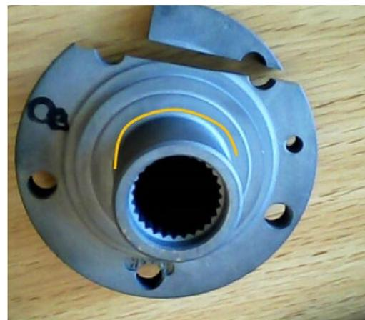
**Fig.3** - Real image of the wheel's hub after nitriding and sample cutting for metallographic analysis. The yellow line shows the notch area subjected to induction hardening and shot peening.
