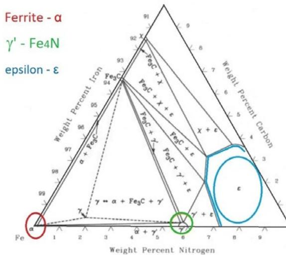
**Fig.1** - Metastable Fe-C-N diagram isothermal section at 565 °C [8]. In the evidenced colored areas, there are shown the fields of existence of the ferrite, Fe<sub>4</sub>N- $\gamma'$  and epsilon phases respectively.
