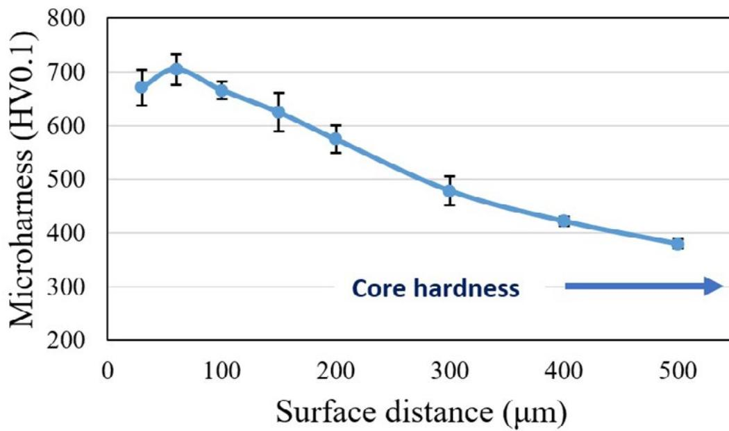
Fig.7 - Low pressure nitriding microhardness profile and standard deviation ranges (HV 0.1).
