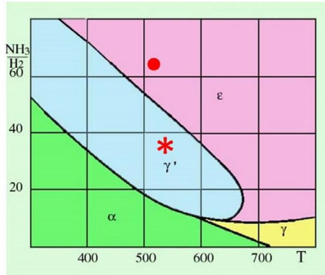
**Fig.4** - Lehrer diagram for  $NH_3 - H_2$  gas mixtures in equilibrium with solids of the Fe-N system ( $P = 1$  bar). On the diagram the nitriding potential conditions for the first (•) and second (\*) stage in case of conventional nitriding treatment are reported.
