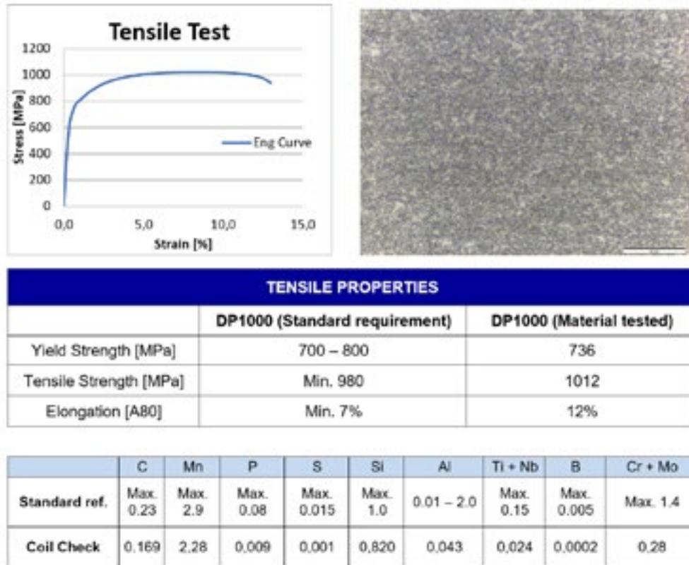
**Fig.4** - Mechanical properties, chemical composition and microstructure of DP1000
