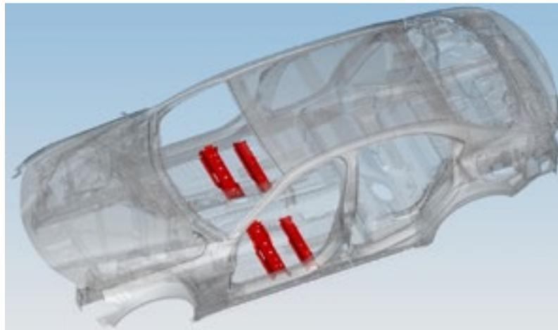
**Fig.2** - Under-seats beam position on the vehicle
