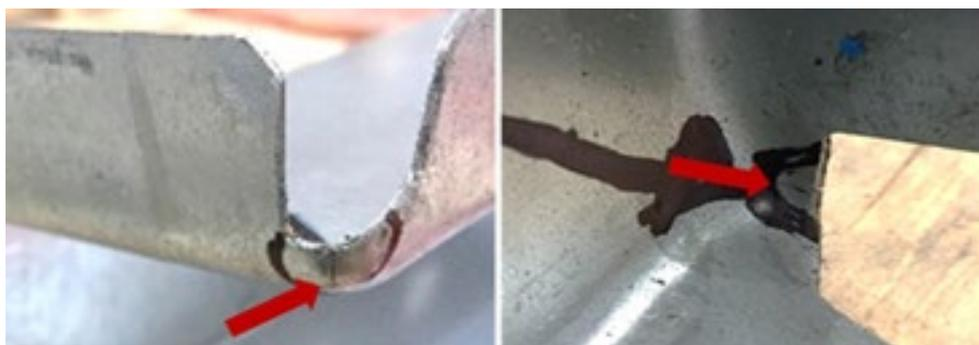
**Fig.3** - Cracks during the forming operations.
