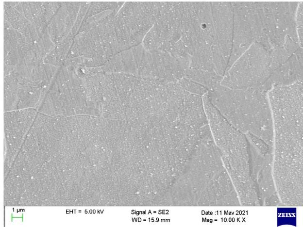
**Fig.6** - SEM image of 300-grade maraging steel after SAT + Q heat treatment.
