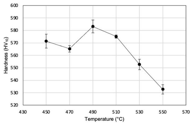
**Fig.7** - Values of hardness (HV<sub>10</sub>) in relation with temperature (aging time: 6 hours).
