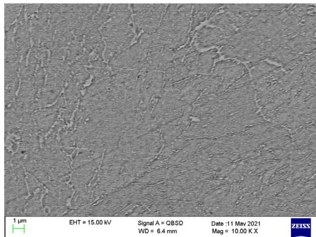
**Fig.10** - SEM image referred to the worst condition of AHT (550 °C, 6 h).
