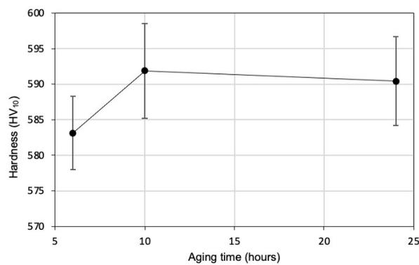
**Fig.8** - Effect of aging time on hardness (treatment temperature: 490 °C).
