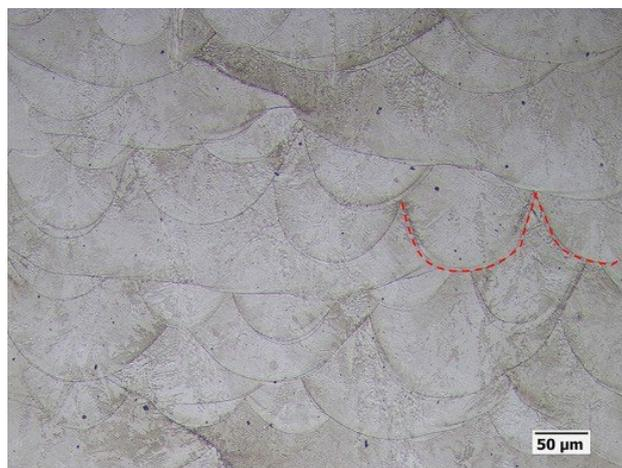
**Fig.3** - OM image of 300-grade maraging steel as-built sample. The red dotted lines delineate the of the melt pools.
