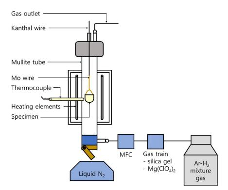
Fig.2 - Schematic presentation of experimental apparatus for hydrogen solubility measurements.
