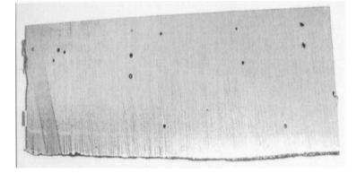
Fig.1 - Photograph of pin-hole defect just under the surface of martensitic stainless steel product.
