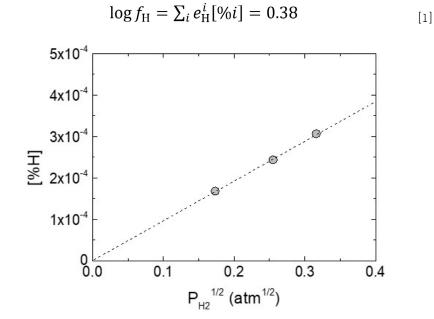
Fig.3 - Relationship with H2 partial pressure and hydrogen content in molten stainless steel.
