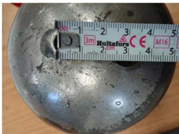
**Fig.3** - installation position of the FOPS (hole to the right) seen relative to the argon injection hole (to the left).
