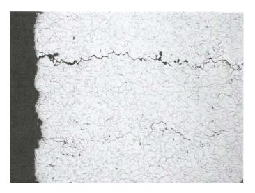
Fig.1 - Intergranular stress corrosion cracking of carbon steel in industrial grade methanol (X Nital) /
