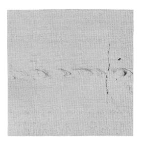
**Fig.6** - Stress corrosion cracking observed on a welded vessel used as a storage for industrial grade methanol / Tensocorrosione rilevata in un serbatoio di metanolo.
