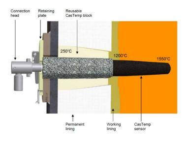
Fig.4 - Cross section of Tundish showing temperature profile.
