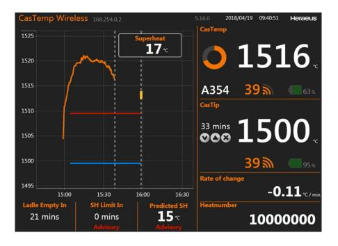
Fig.5 - CasTemp Superheat Operator Display.
