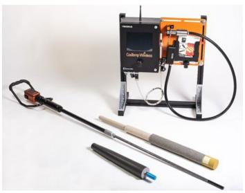
Fig.3 - Equipment for CasTemp Superheat.
