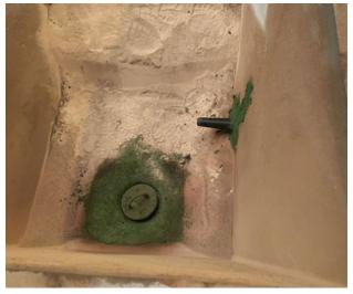
**Fig.5** - CasTemp Sensor Installed in a Tundish.
