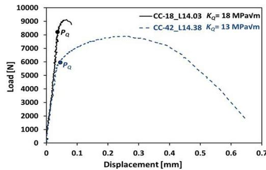
**Fig.3** -  $P_Q$  determination from load-displacement curves of Castaduct-18 and Castaduct-42.
