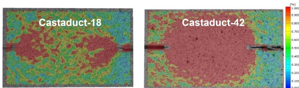
**Fig.5** - DIC measurements of the plastic zone ahead of the crack tip for the two studied alloys.
