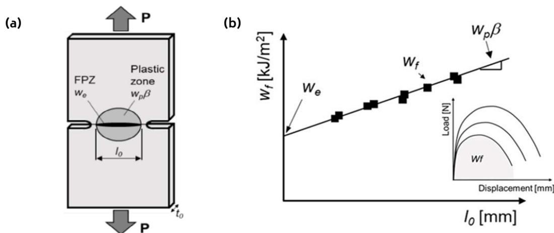
**Fig.2** - (a) DENT specimen ;(b) Linear relationship between total specific work and the ligament length and determination of  $w_e$  at the y-axis intercept.
