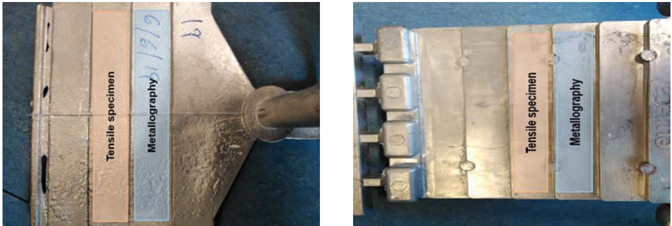
Fig.2 - Images of a PMC part (left) and HPDC part (right) indicating the regions where the specimens for tensile test and metallographic inspection were extracted.
