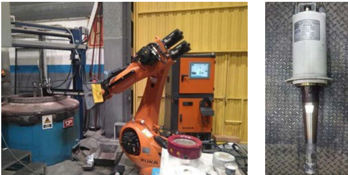
Fig.1 - Experimental set-up used in the experiments, general view of the prototype (left) and detail of the ultrasonic generator and wave-guiding equipment (right).
