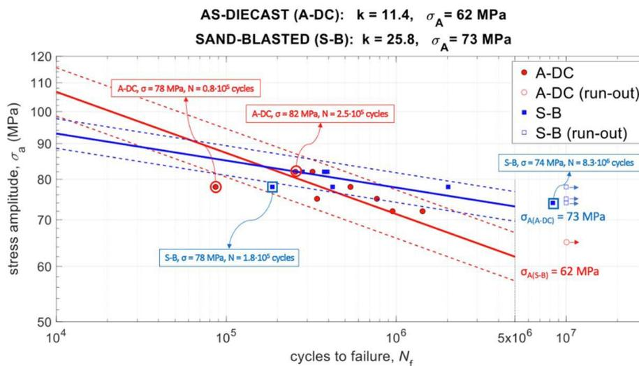
Fig.1 - S-N curves for as-diecast and sand-blasted specimens.
