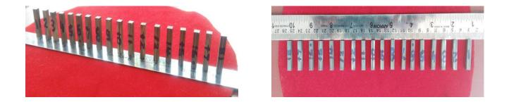
Fig.2 - 18 samples (5 x 5 x 25 mm) after Wire EDM (a) vertical position (b) horizontal
