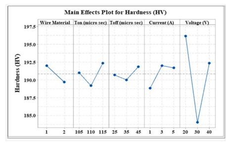
Fig.5 - Main effect plot for microhardness
