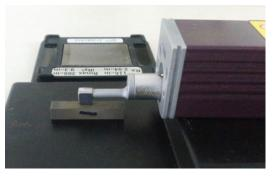
Fig.3 - Surface roughness measurement
