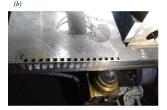
Fig.1 - a. Wire EDM facility. b. machining of SS 304 Workpiece
