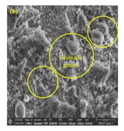
Fig.6 - Microstructure of the machined surface (a) 5<sup>th</sup> experiment with Zn coated brass wire (b) 13<sup>th</sup> experiment with uncoated brass wire.
