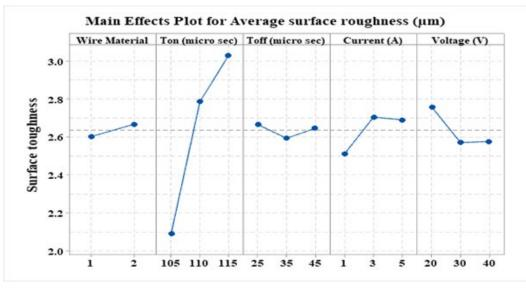
**Fig.4** - Main effect plot for surface roughness
