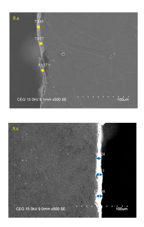
Fig.8 - Recast layer thickness of the machined samples (a) for Exp. no. 1 – average RLT-8.069 μm (b) Exp. no. 7– average RLT-14.815 μm (c) Exp. no. 13– average RLT-10.714 μm.
