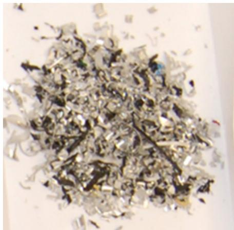
**Fig.1** - Filter dust from shredding aluminium profiles.
