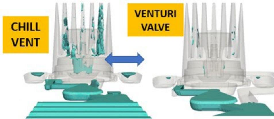
**Fig.9** - Entrapped air without and with the use of Venturi valve.
