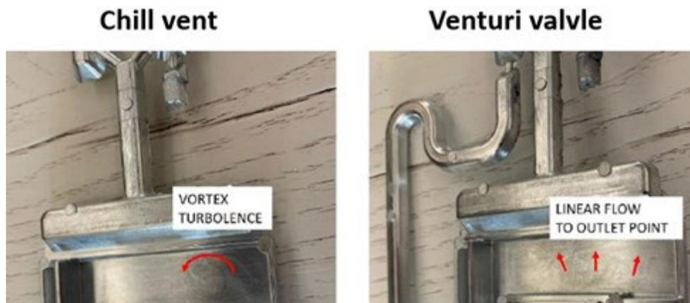
**Fig.10** - Flow in real casting (ZAMAK).
