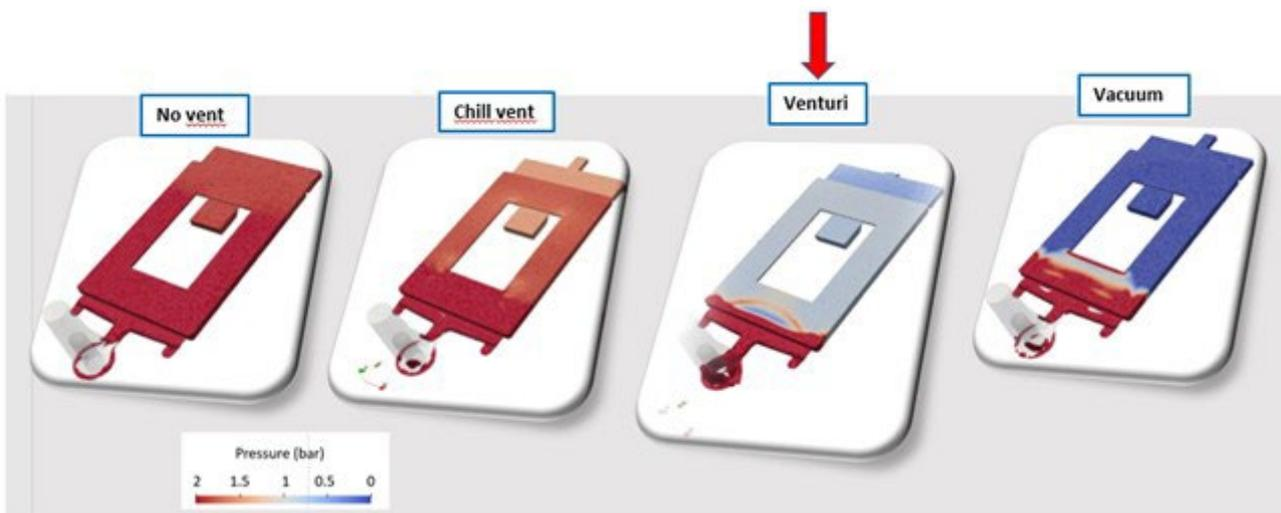
**Fig.2** - Comparison with other technology (air pressure in cavity).
