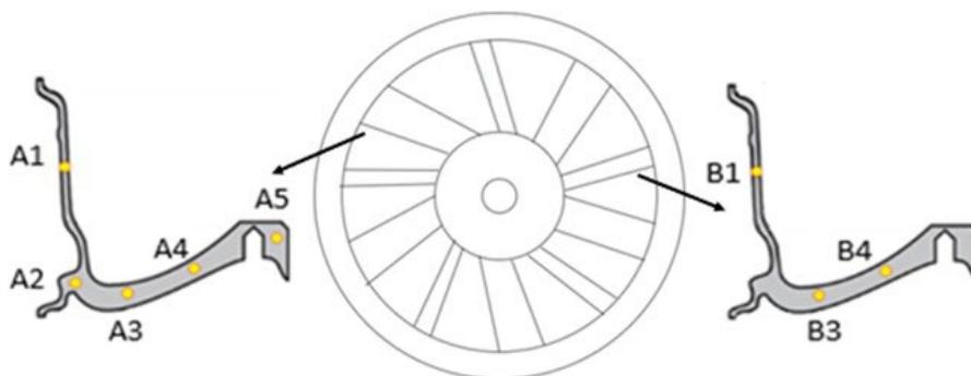
**Fig.1** - Schematic representation of samples drawn from the two different spokes. For confidentiality reasons, the real wheel cannot be shown so a schematic representation is given.
