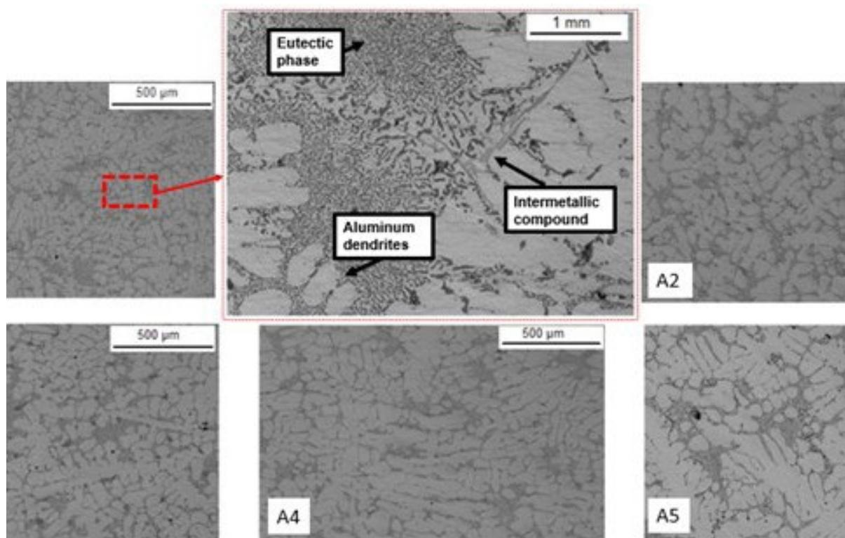
**Fig.2** - Microstructure of each as cast sample. The central in-set shows the main microstructural constituents.
