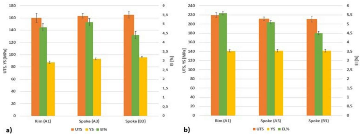
**Fig.3** - Tensile properties from as-cast (a) and T6 (b) wheels.
