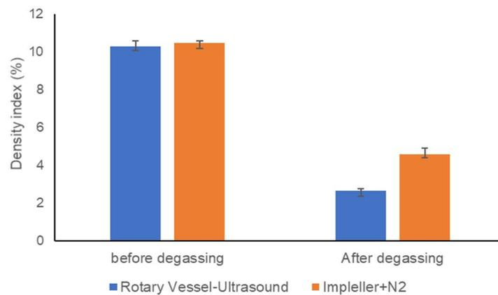
**Fig.2** – Density index of molten metal before and after degassing with two different methods.
