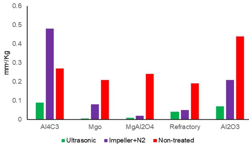
**Fig.3** – PoDFA analysis of untreated, impeller+N<sub>2</sub> and ultrasonically treated melts.
