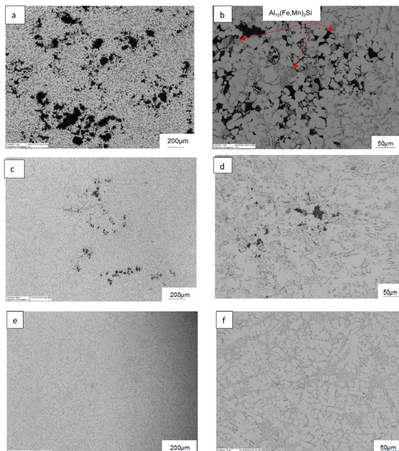
**Fig.4** – Microstructure of diecast AlSi<sub>9</sub>Cu<sub>3</sub>(Fe) alloy: (a,b) untreated; degassed with (c,d) impeller+N<sub>2</sub> and (e,f) rotary vessel-sonication.
