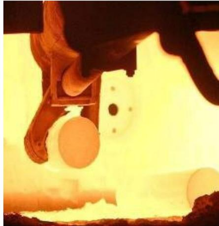
**Fig.2** - Round billets for tube production being heated before piercing using Flameless Oxyfuel in a Rotary Hearth Furnace at ArcelorMittal in the USA. Here the conversion from air-fuel resulted in fuel savings of 60%..
