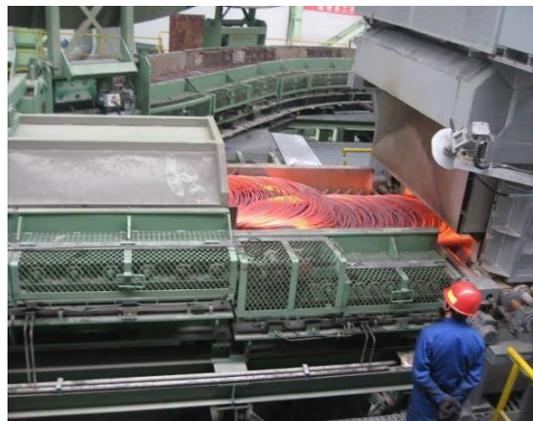
**Fig.4** - Coiled wire rod entering a REBOX DST line operating 100% with Flameless Oxyfuel at Yongxing, China, providing the world's lowest fuel consumption for stainless wire rod annealing.
