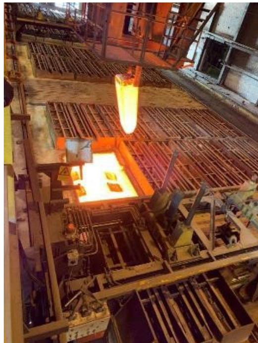
**Fig.7** - The world's first full-scale reheating of steel with 100% hydrogen as fuel, using REBOX Hyox Flameless Oxyfuel, at Ovako's Hofors mill in Sweden in March 2020.
