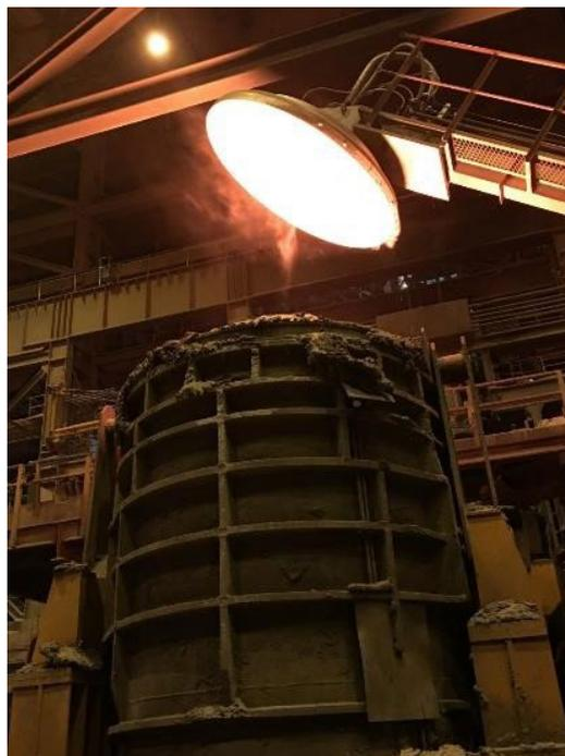
**Fig.3** - OXYGON Flameless Oxyfuel ladle preheating at Taiwanese stainless steel producer Walsin.
