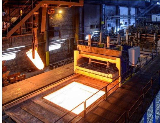
**Fig.5** - Discharging of a stainless steel ingot from soaking pit furnace at Sandvik, Sweden, operation with 100% Flameless Oxyfuel.
