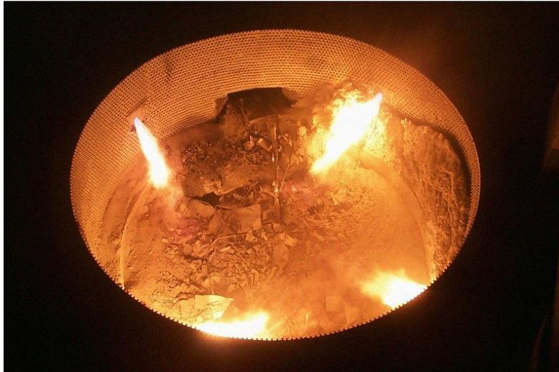
**Fig.1** - Four Cojet injectors in operation in an EAF.
