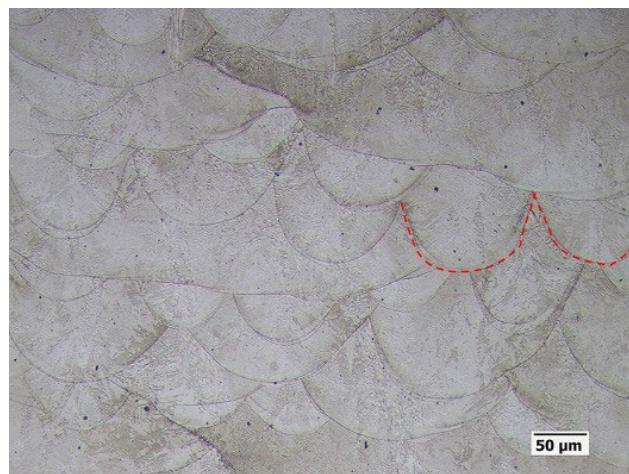
**Fig.3** - OM image of 300-grade maraging steel as-built sample. The red dotted lines delineate the melt pools.
