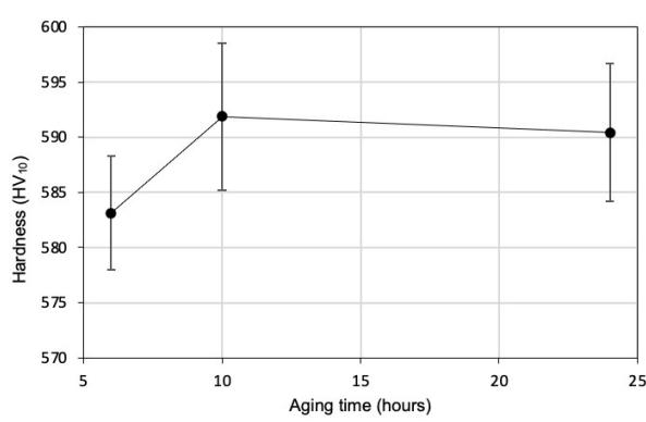
**Fig.8** - Effect of aging time on hardness (treatment temperature: 490 °C).
