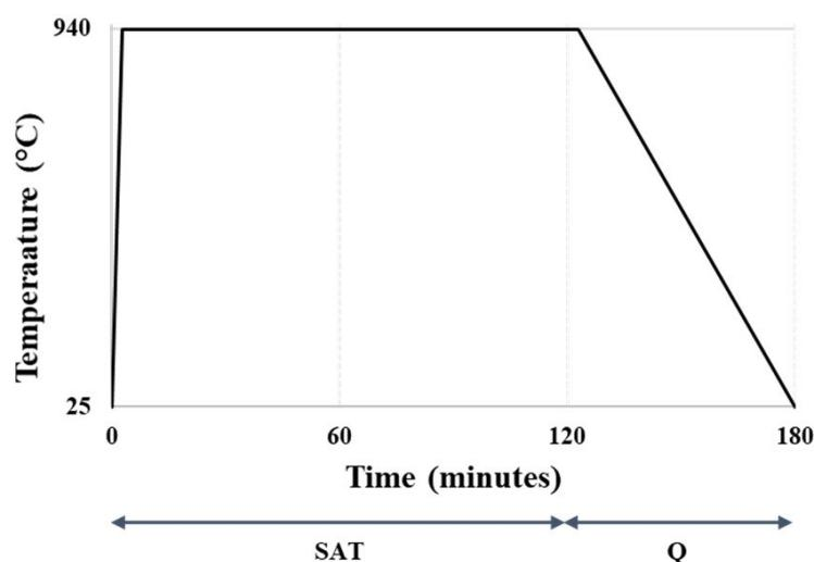
**Fig.1** - Heat profile (SAT + Q).
