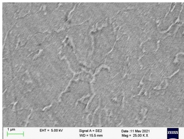
**Fig.9** - SEM image referred to the best condition of AHT (490°C, 6 h).
