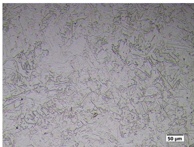
**Fig.5** - OM image of 300-grade maraging steel after SAT + Q heat treatment.
