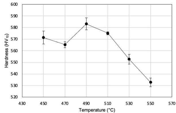
**Fig.7** - Values of hardness ( $\text{HV}_{10}$ ) in relation with temperature (aging time: 6 hours).
