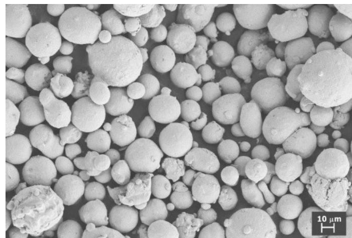
**Fig.2** - SEM image of morphology of 300-grade maraging steel powder.
