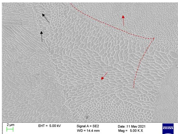
**Fig.4** - SEM image of 300-grade maraging steel as-built sample. The columnar and cellular solidification structures are clearly visible.
