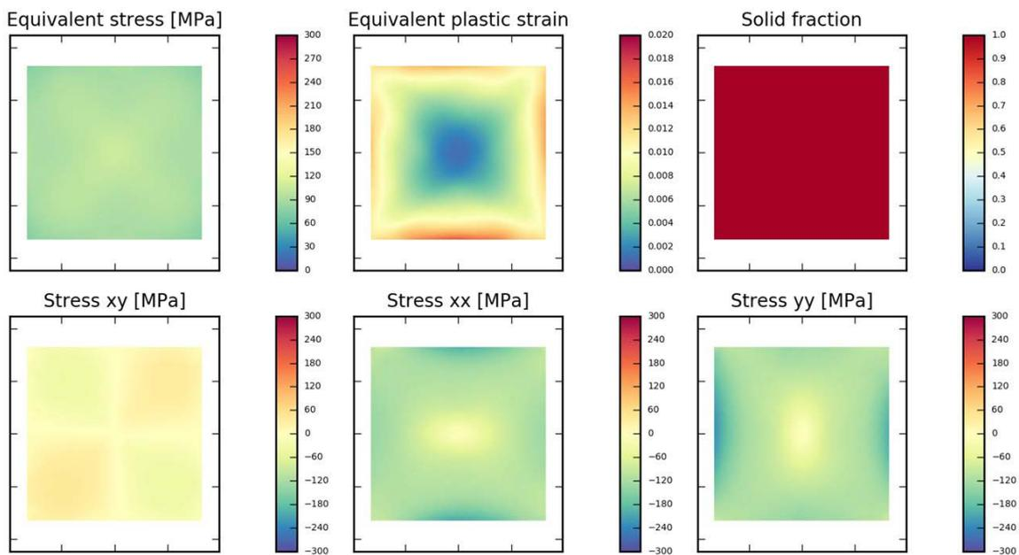
**Fig.6** -The results of the mechanical model at the end of solidification.
