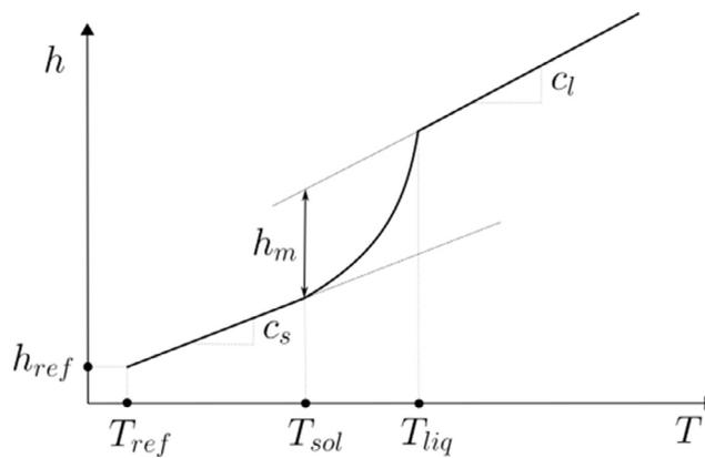
**Fig.1** - The enthalpy as a function of temperature in a binary alloy.
