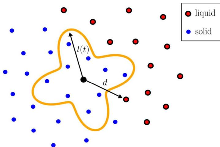
**Fig.2** - A scheme of the PA algorithm for the simulation of grain growth.
