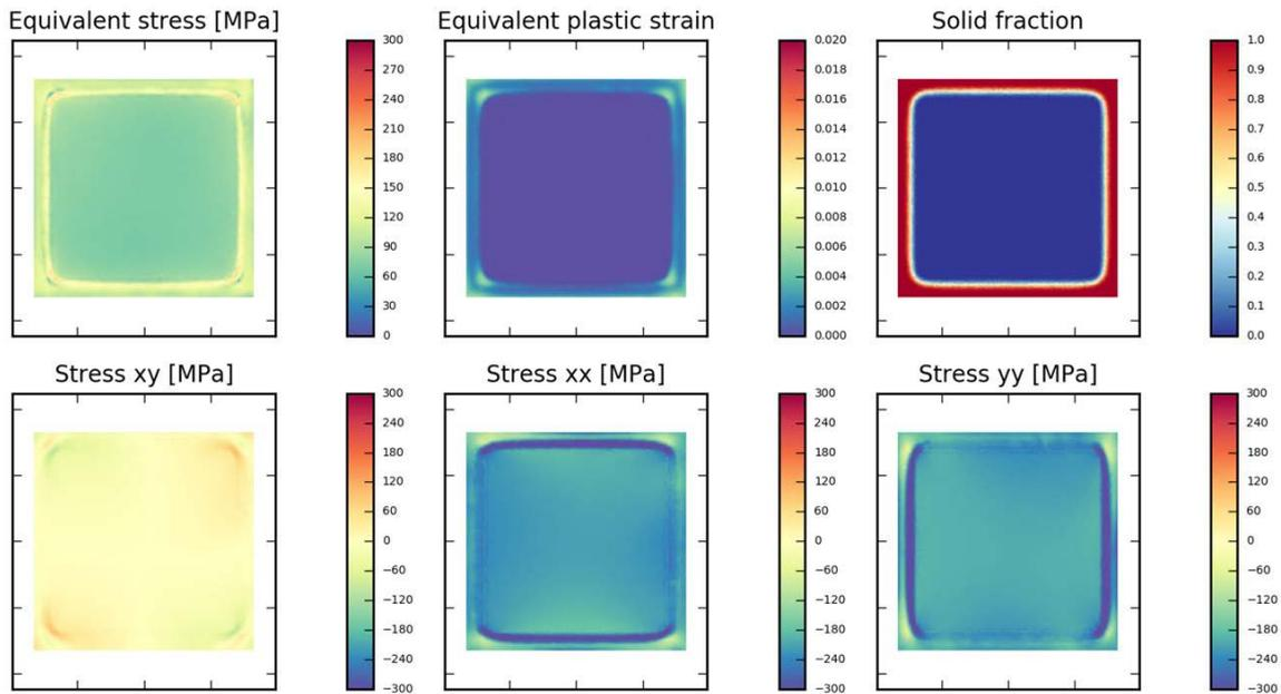
**Fig.5** -The results of the mechanical model at the exit from the mould cooling area.
