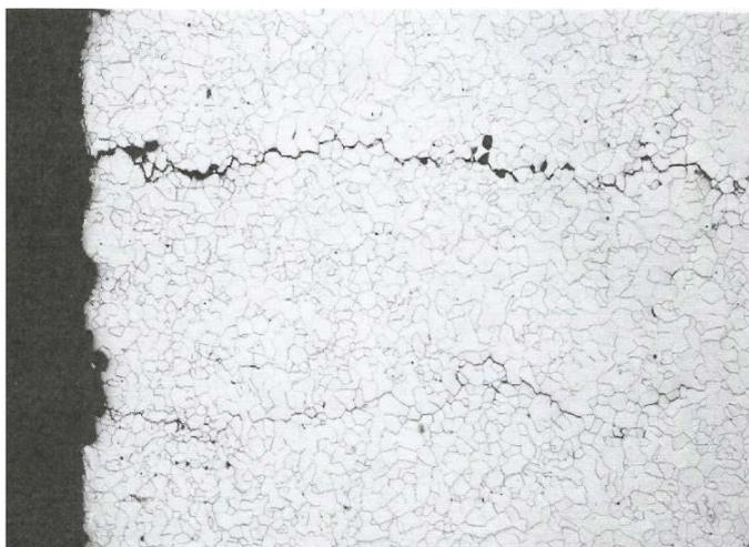
**Fig.1** - Intergranular stress corrosion cracking of carbon steel in industrial grade methanol (X Nital) / Tensocorrosione intergranulare dell'acciaio al carbonio in metanolo industriale (X Nital).
