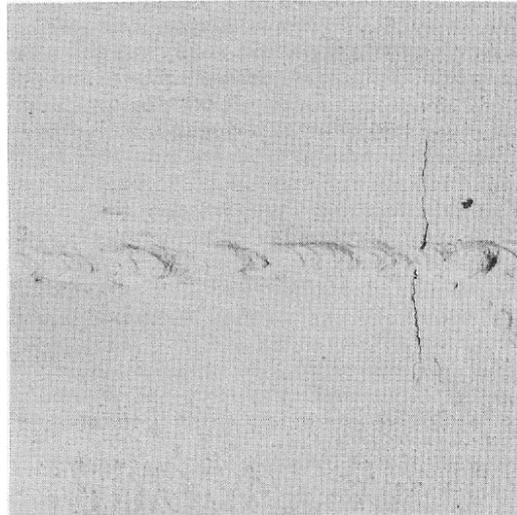
**Fig.6** - Stress corrosion cracking observed on a welded vessel used as a storage for industrial grade methanol /
