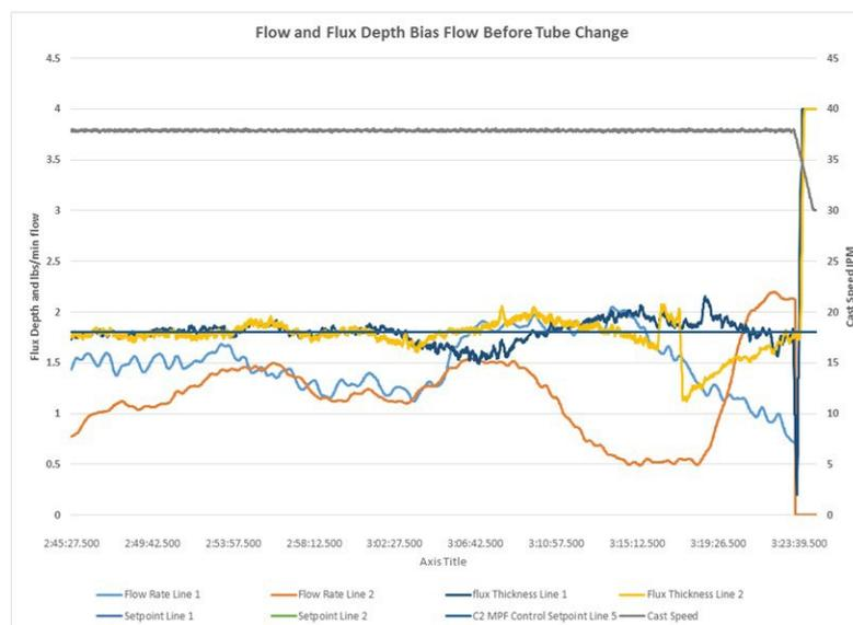
**Fig.4** - At steady state speed (grey) and flux thickness (yellow and dark blue), a bias flow condition occurs prior to a tube change. During the bias flow event, a 4:1 difference of mold flux consumption was measured.
