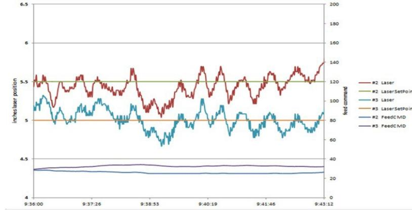
**Fig.1** - The lasers (red and light blue) and feeding signals (purple and dark blue) are displayed on the chart. The setpoint distance for each laser (orange and green) are followed for control of the mold flux thickness. The trend is monitored over 1/2 hr, using a laser scale of +/- 1.25 inches. The agreement of the magnitude and behavior of the laser signals demonstrates the presence of mold level fluctuations.
