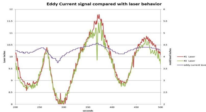
**Fig.2** - During an unstable mold event capture for 300 seconds, the lasers (red and green) were recording the actual mold level variation. The customer mold level signal (purple) is on the same scaling and followed the same trend, but with a filtered response not representing the true mold level fluctuations.
