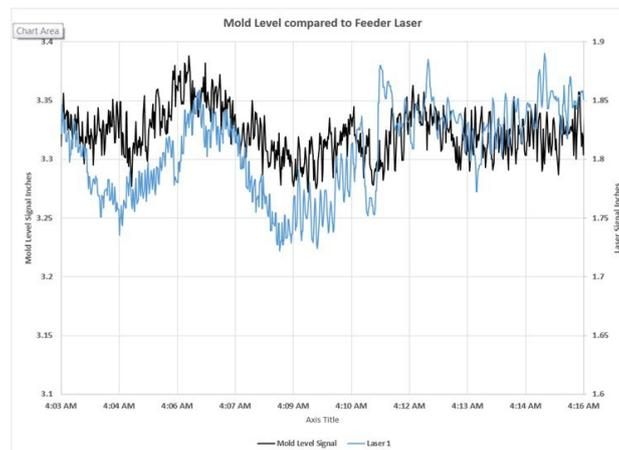
**Fig.3** - The graph shows good agreement in signal behavior and amplitude fluctuation. between the laser signal (blue) and the mold level (black) on the same scale range, giving confidence to the mold level control performance.
