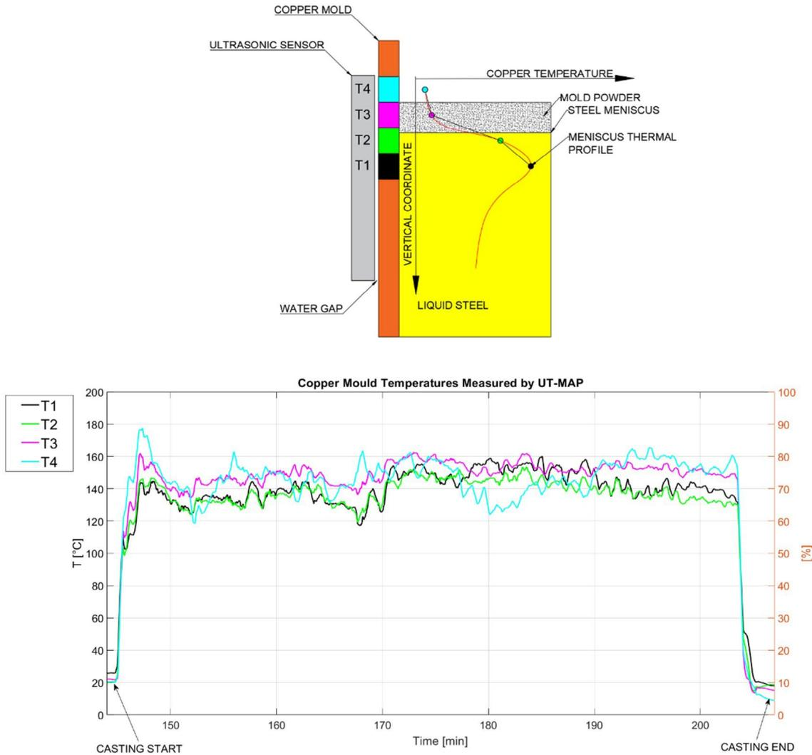
**Fig.5** - Example of copper temperature data measured by the ultrasonic sensor: The location where each temperature is measured is represented in the diagram above the graph.
