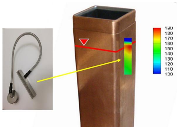
**Fig.4** - Schematic representation of a typical UT-MAP measuring area: Copper temperature is mapped vertically in the meniscus region
