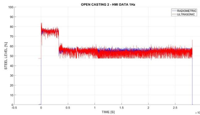
**Fig.6** - Comparison of ultrasonic (red) and radiometric sensor (blue). Steel level was controlled by radiometric and measured with ultrasonic sensor (HMI unfiltered raw data sampled at 1 Hz).
