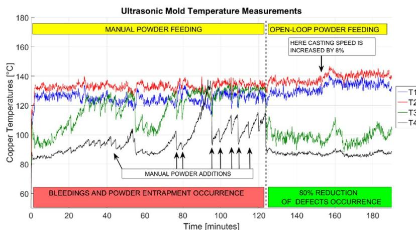
**Fig.8** - UT-MAP trends detect difference between manual feeding, leading to defects occurrence on tracked billets, and automatic feeding (open-loop), leading to marked defect reduction<sup>6</sup>.
