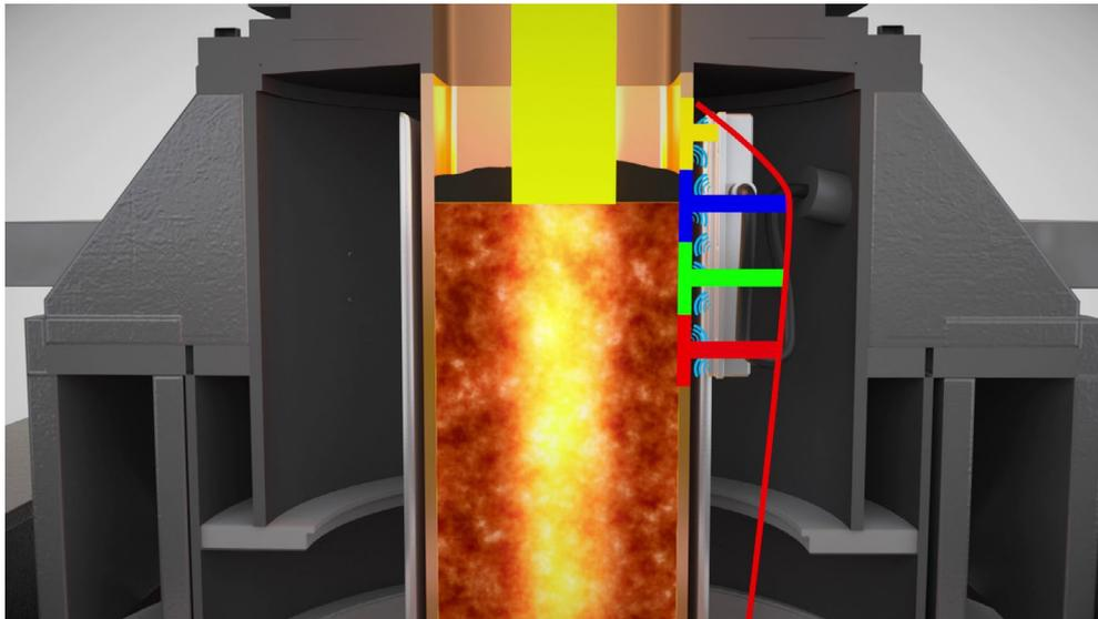
**Fig.3** - Concept of ultrasonic temperature measurement: 1) Ultrasound propagates through the water gap and along the mold wall; 2) signal processing converts the ultrasonic signals into copper temperatures (colored beams); 3) the meniscus thermal profile is reconstructed (red line).
