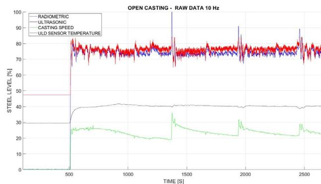
**Fig.7** -Comparison between ULD and radiometric level signals. Steel level was controlled by radiometric and measured with ultrasonic sensor. Open casting with clogging events.
