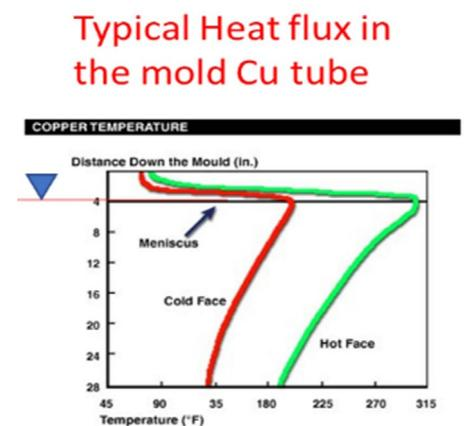
**Fig.1** - Simulation of heat flux in the mold and temperature step response inside a copper tube.
