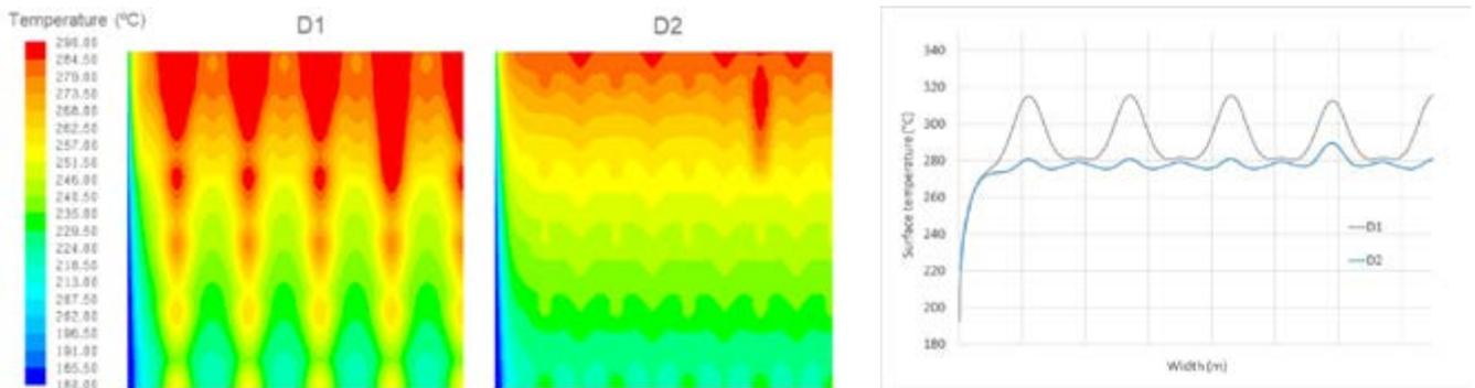
**Fig.9** - Effect of plate design on broad face temperature (Left) and on temperature profile along width (Right) depending on plate design.
