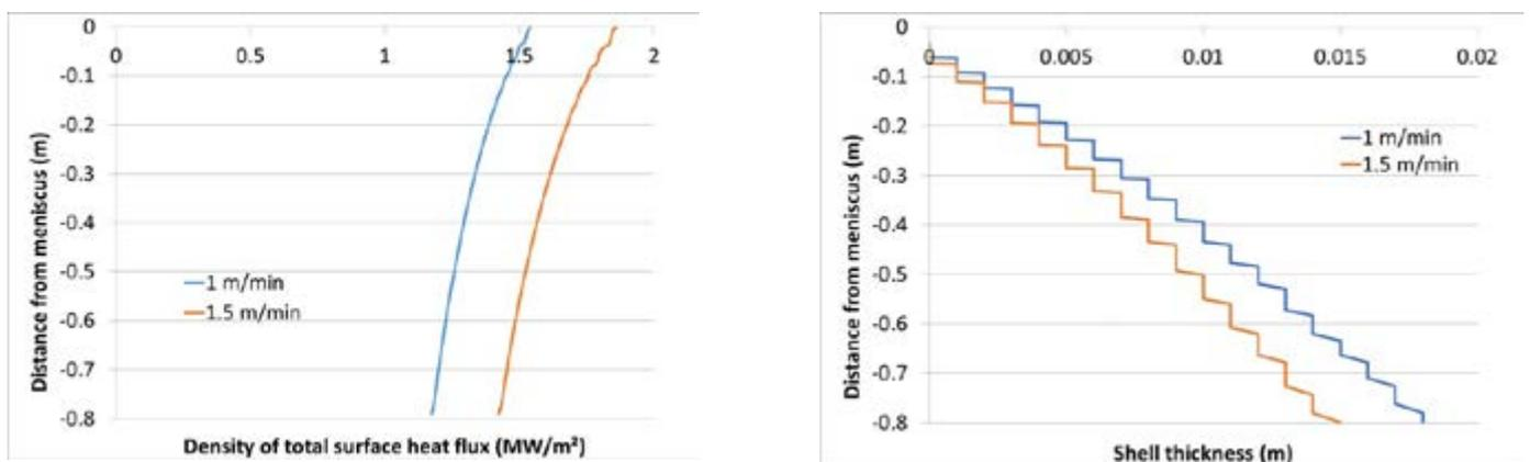
**Fig.3** - Effect of casting speed on extracted heat flux (Left) and on solidified shell thickness (Right) along the mould height on broad face.
