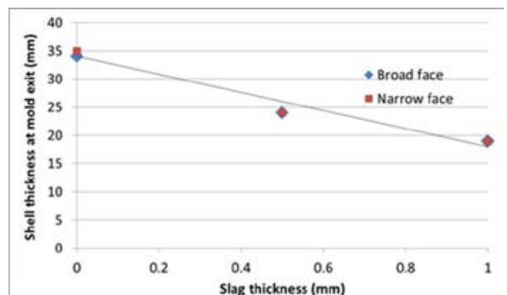
**Fig.2** - Effect of infiltrated slag thickness on heat flux extraction (Left) and on solidified shell thickness (Right).
