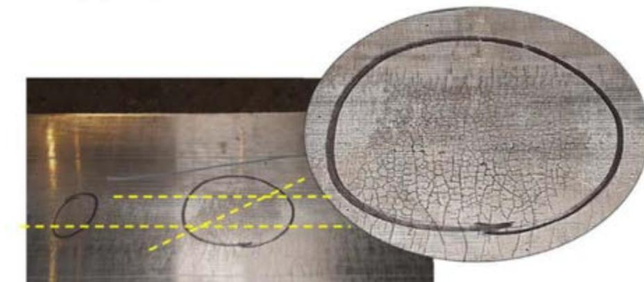
**Fig.6** -Ni coating damage on broad face.
