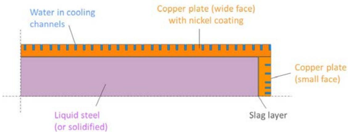
**Fig.1** - Geometry used in the CFD model (top view).
