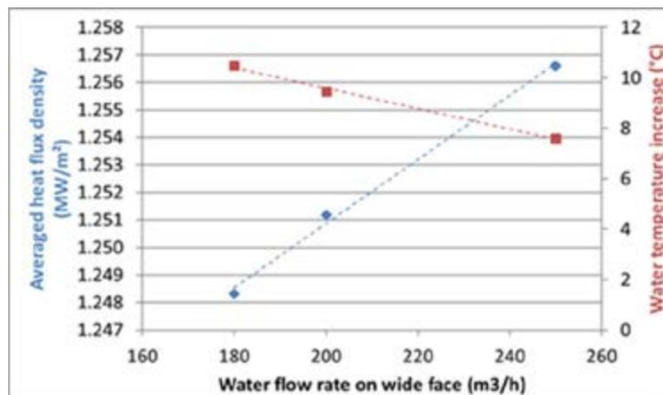
**Fig.4** - Effect of cooling water flow rate on extracted heat flux and on water temperature increase.
