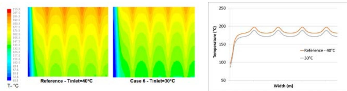
**Fig.6** -Effect of inlet cooling water temperature on broad face temperature distribution (Left) and profile along the mould width (Right).
