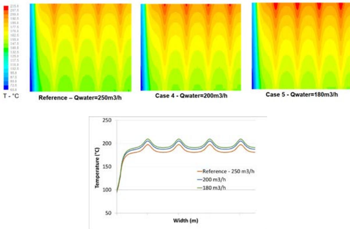
**Fig.5** - Effect of cooling water flow rate on broad face temperature distribution (Up) and temperature profile along the mould width (Down).
