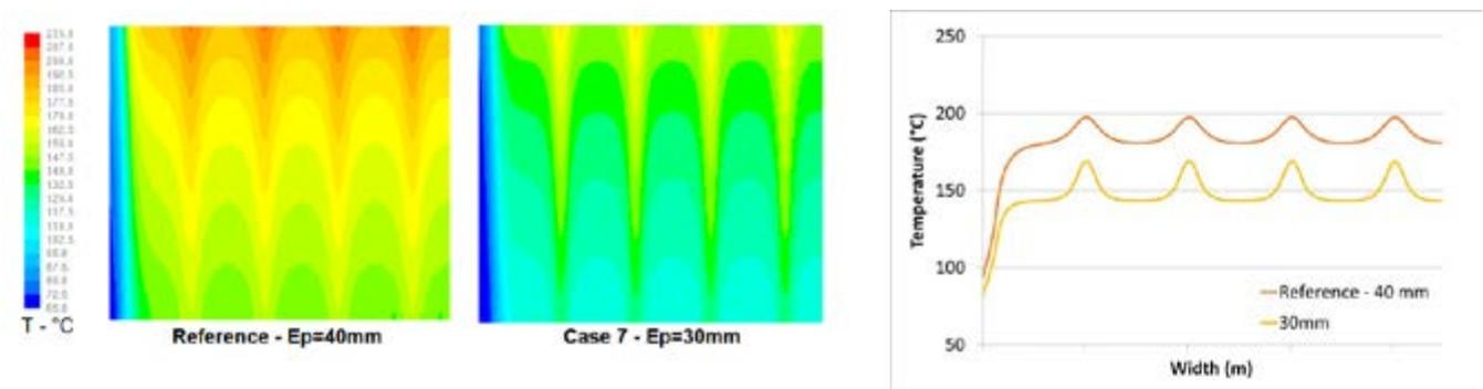
**Fig.7** - Effect of copper broad face thickness on broad face temperature distribution (Left) and along the mould width (Right).
