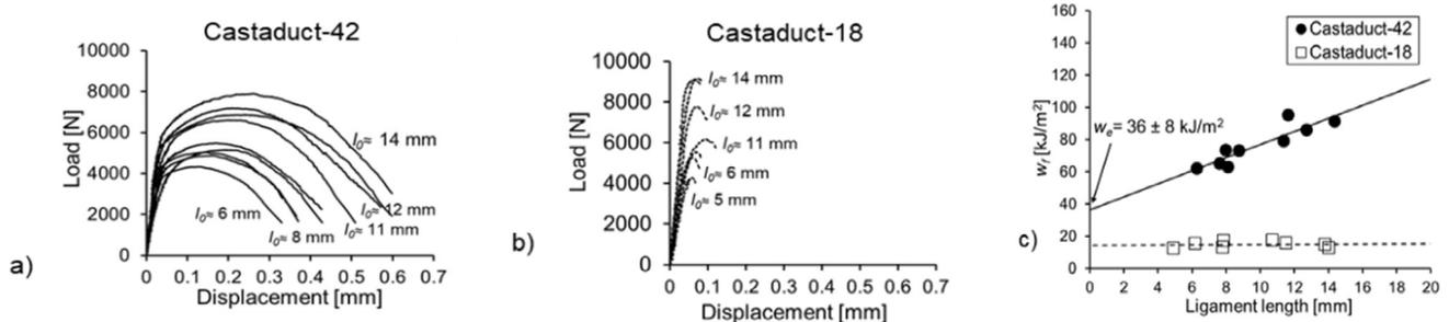
**Fig.4** - Load-displacement curves and EWF for Castaduct-18 and Castaduct-42.
