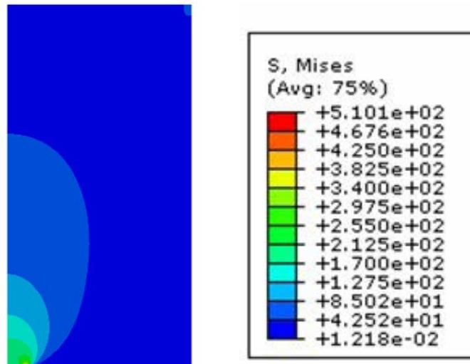
**Fig.6** - Von Mises stress distribution at the crack tip.
