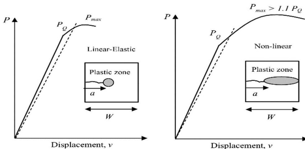
**Fig.1** -  $P_Q$  determination as described in ASTM-E399.
