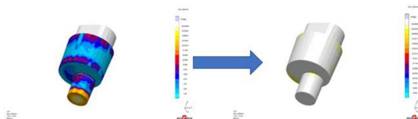
**Fig.3** - Die life results improvement: on the left conventional design on the right conformal cooling design, showing a much longer die life duration through the colors on the top of the scale representing the number of cycles.
