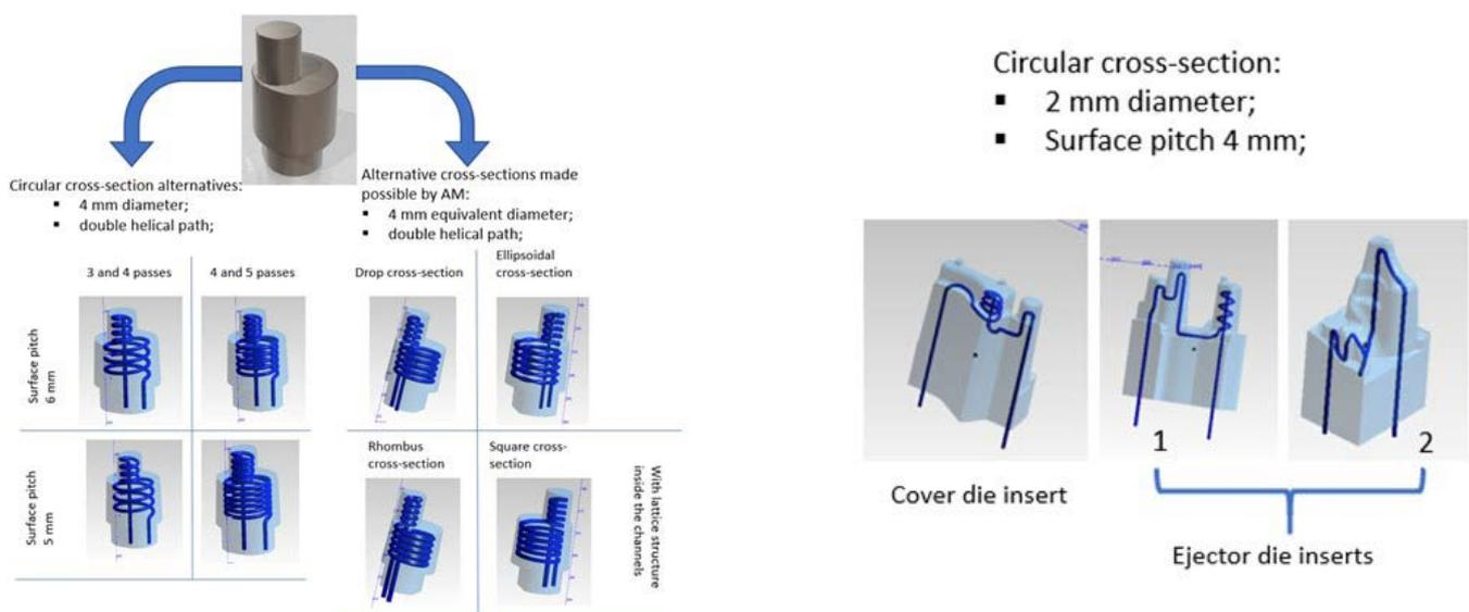
Fig.1 - Conformal cooling proposed designs.
