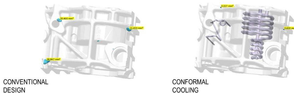
**Fig.2** - Critical porosities reduced using conformal cooling.
