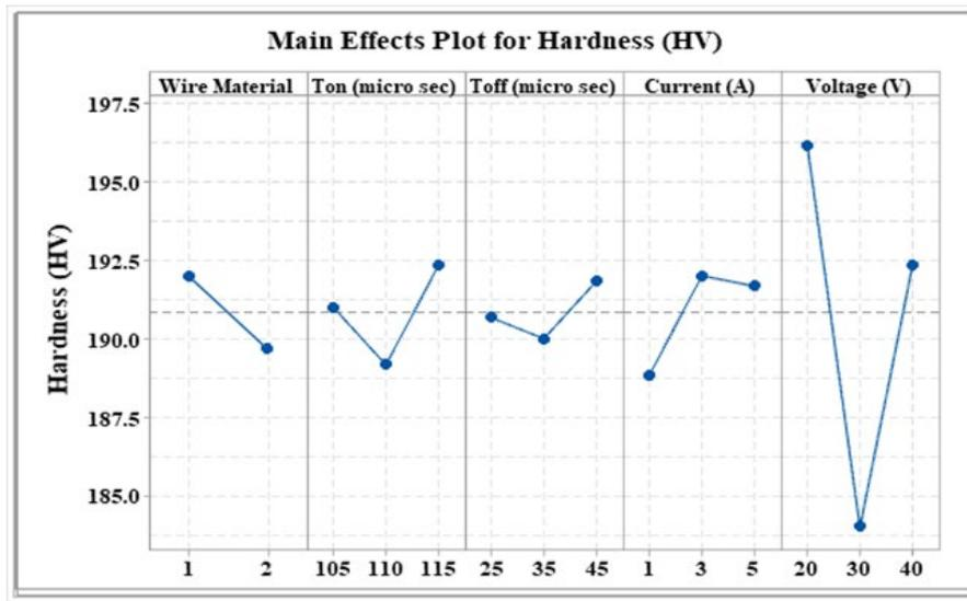
**Fig.5** - Main effect plot for microhardness
