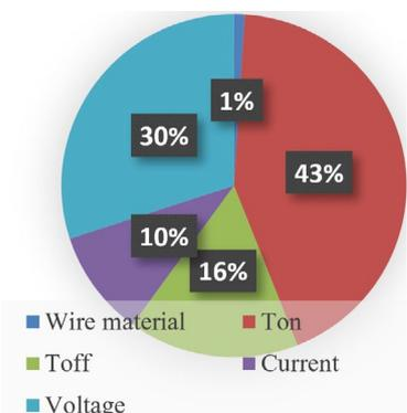
From the table 4 and figure 9 (Pie chart), the most influencing factor for the both minimization of surface roughness and maximization of hardness is identified as Ton (43%) and Voltage (30%).
