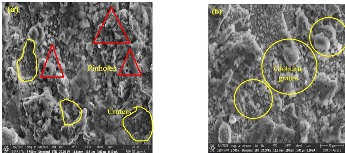
**Fig.6** - Microstructure of the machined surface (a) 5<sup>th</sup> experiment with Zn coated brass wire (b) 13<sup>th</sup> experiment with uncoated brass wire.
