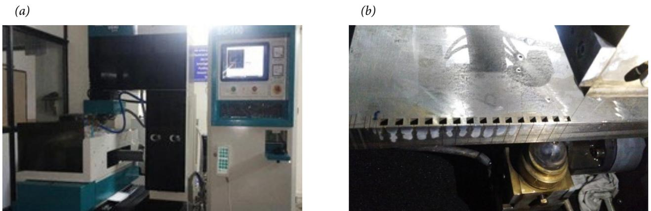
**Fig.1** - a. Wire EDM facility, b. machining of SS 304 Workpiece
