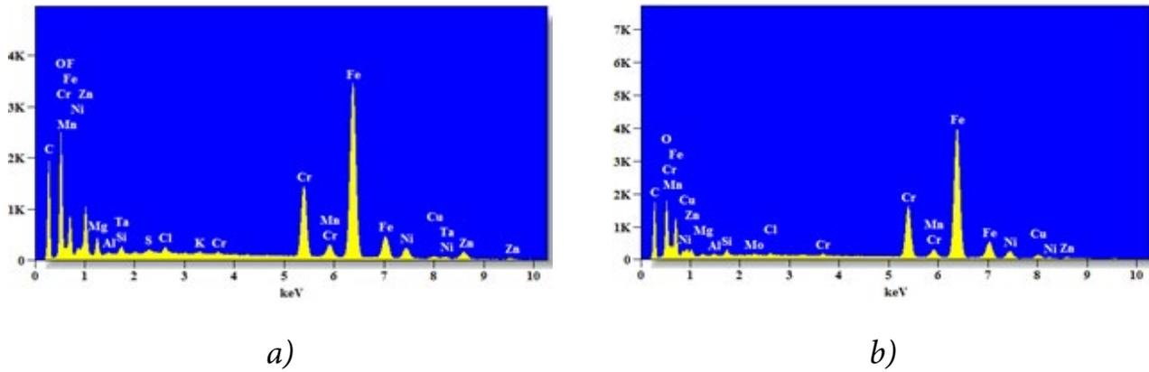
**Fig.7** - Energy Dispersive X-ray (EDX) analysis (a) 5<sup>th</sup> experiment (b) 13<sup>th</sup> experiment.
