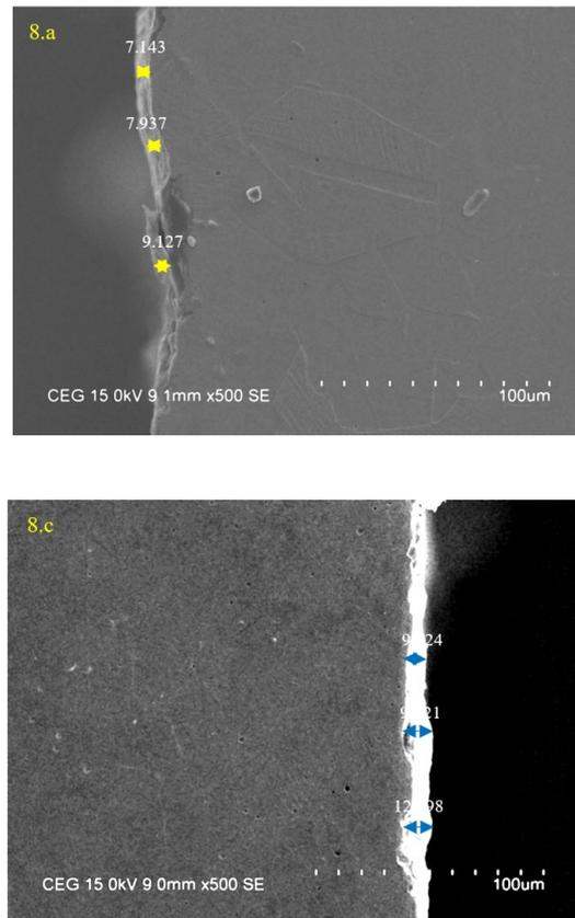
**Fig.8** - Recast layer thickness of the machined samples (a) for Exp. no. 1 – average RLT-8.069  $\mu\text{m}$  (b) Exp. no. 7– average RLT-14.815  $\mu\text{m}$  (c) Exp. no. 13– average RLT-10.714  $\mu\text{m}$ .
