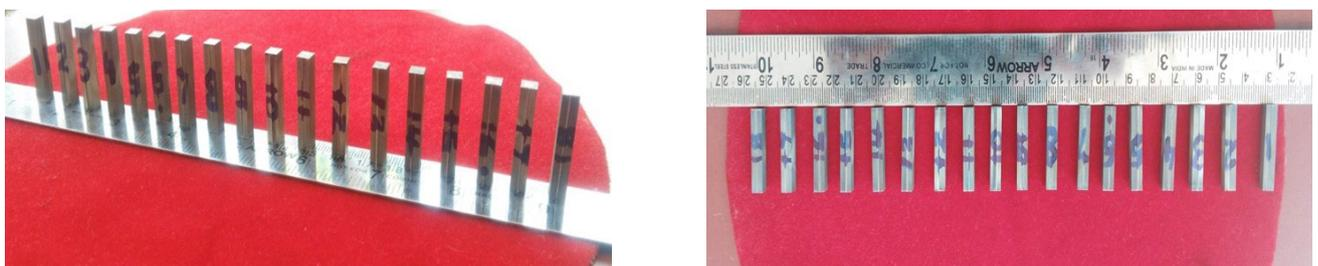
**Fig.2** - 18 samples (5 x 5 x 25 mm) after Wire EDM (a) vertical position (b) horizontal
