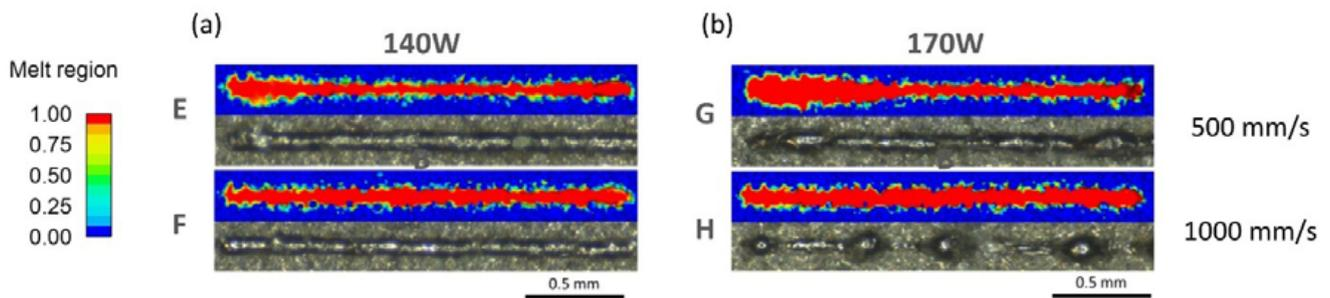
**Fig.3** Comparison between simulation and experimental results of track morphology, with 90  $\mu\text{m}$  of layer thickness and with (a) 140 W and (b) 170 W of laser power, see Table 1 for further process parameters.
