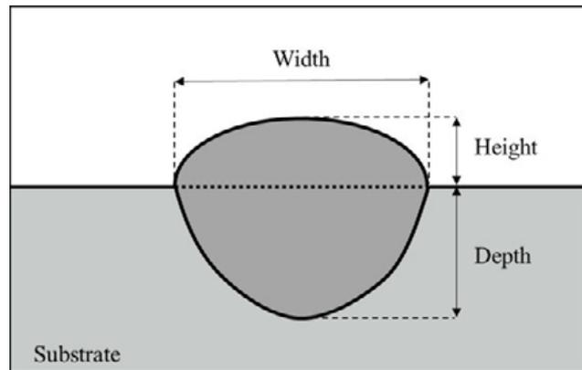
**Fig.4** Schematic representation of size measurements for the cross section of melt pool.
