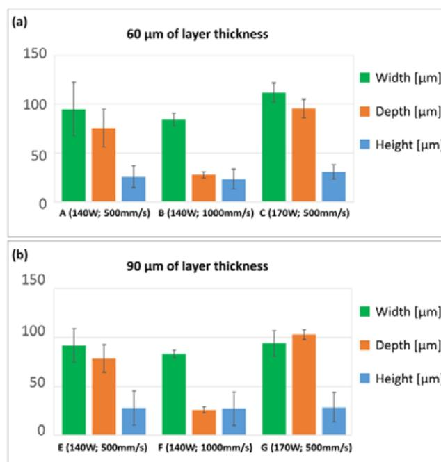
**Fig.5** Melt pool measures (and corresponding standard deviation) for simulated tracks in agreement with real tracks, in the cases of a layer thickness of (a) 60 μm and (b) 90 μm
