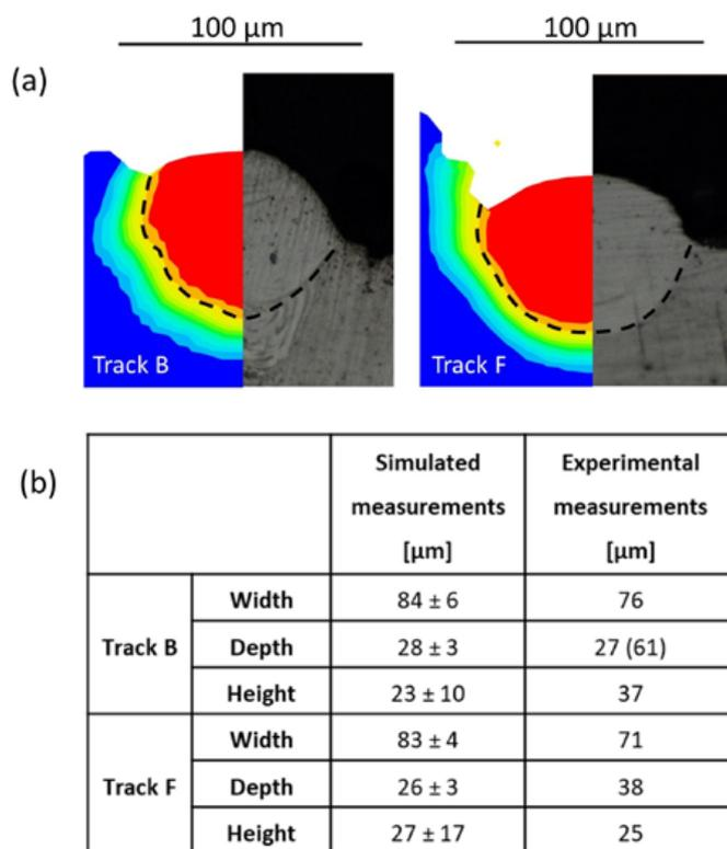
**Fig.7** Simulation and experimental results for track B and F, for (a) shape and (b) dimensions of the melt pool.
