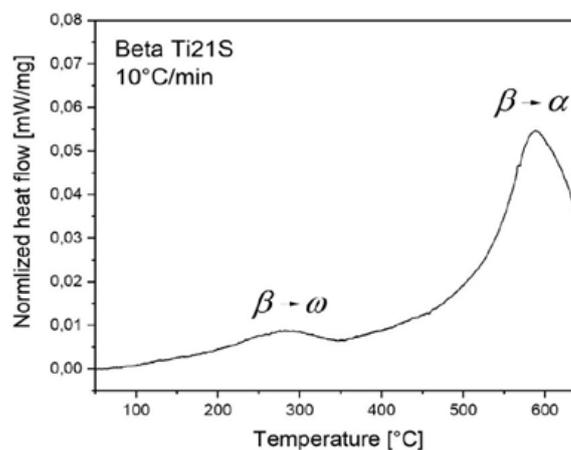
**Fig.3** -DSC curve showing the precipitation of  $\omega$  and  $\alpha$  phase.
