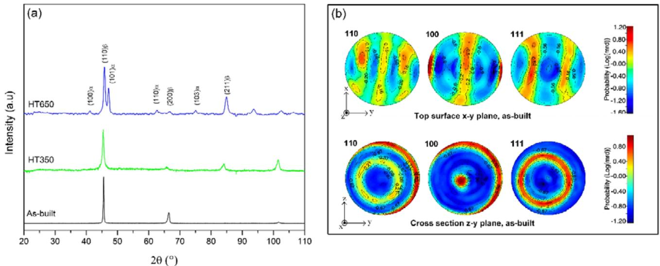
**Fig.4** - (a) phase evaluation during heat treatment, alpha precipitations peaks appeared after 650 °C, (b) pole figures projection from the top and lateral sections of the as-built sample.
