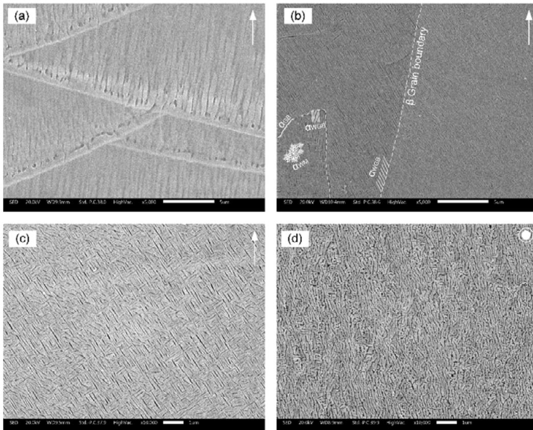
**Fig.5** Micrographs of (a) HT350 (b), (c), and (d) HT650 samples, three types of alpha are shown in the (b).  $\alpha_{WM}$  is shown from top and lateral sections in the (c) and (d). The arrow shows the building direction.
