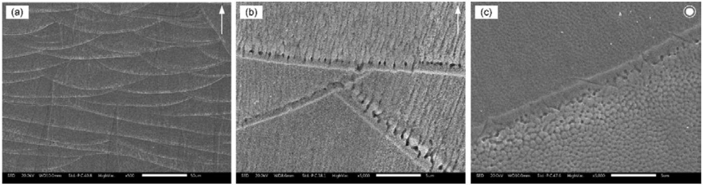
**Fig.2** -Micrographs of (a), (b) Lateral and (c) Top views of as-built microstructure. The arrow shows the building direction.
