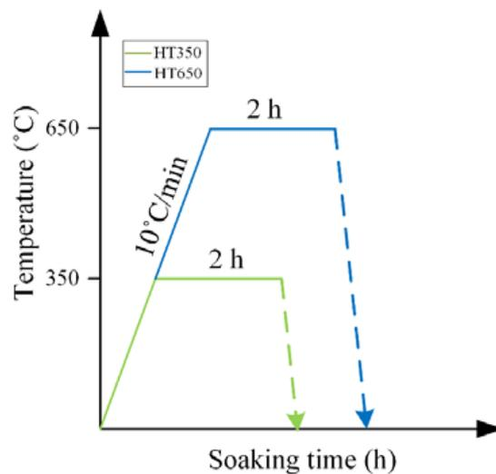
**Fig.1** -The two ageing treatments studied in this work HT350 and HT650.
