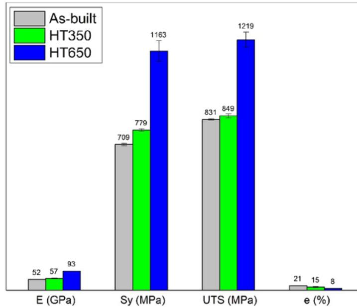
**Fig.6** Mechanical properties resulted from the tensile test. Young modulus (E), Sy (yield strength, Ultimate tensile strength (UTS), and elongation (e).
