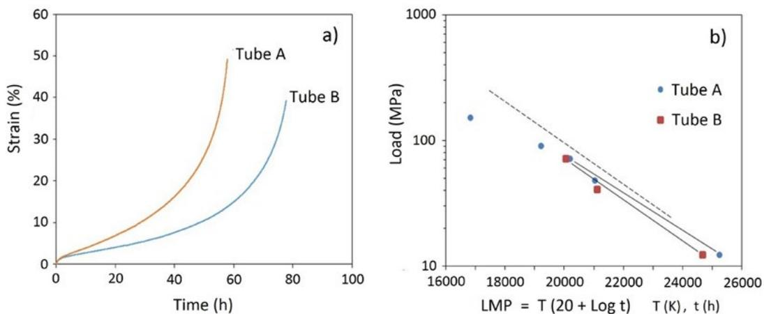
**Fig.4** - Creep curves in comparison obtained at 650°C and 70 MPa (a) and experimental points on the Larson-Miller diagram (b).
