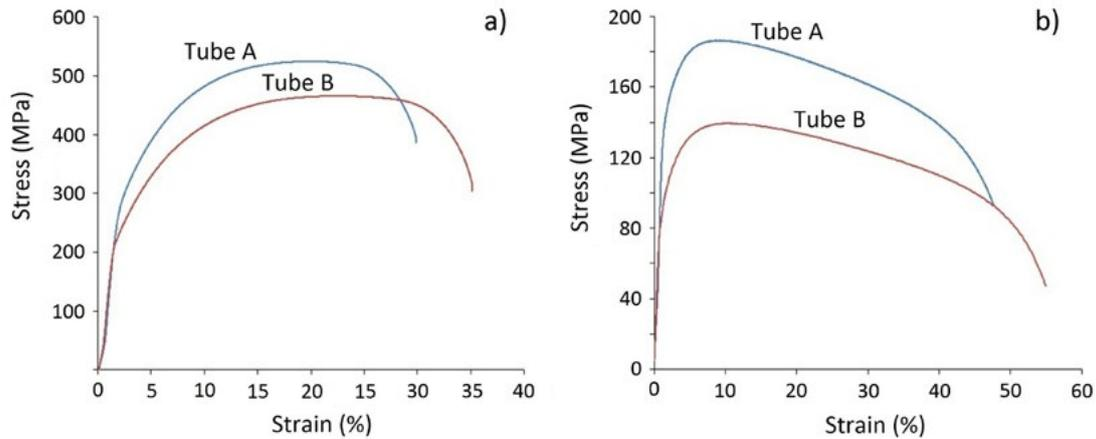
**Fig.3** - Stress-strain curves: a) room temperature, b) T=650°C.
