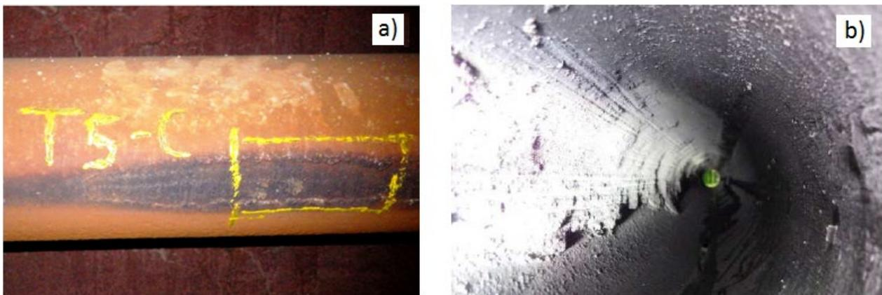
**Fig.1** - External burning (a) and carbon sediment on tube internal surface (b).
