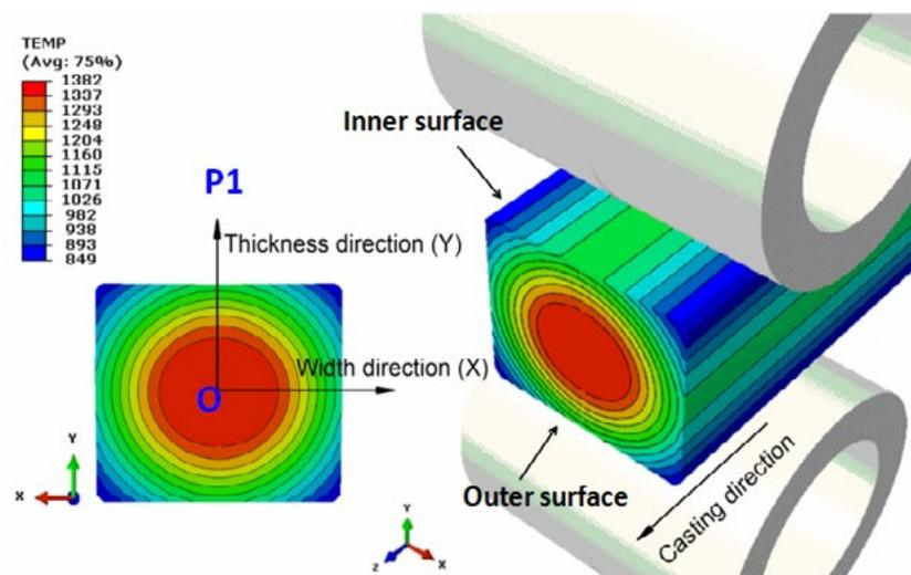
**Fig.1** - Deformation finite element model.
