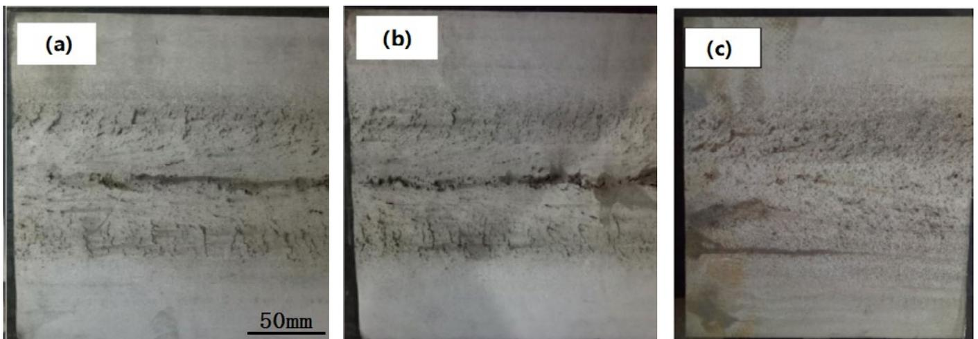
**Fig.10** - Longitudinal morphologies of as-cast bloom under designed experiment cases: (a) case 1; (b) case 2; (c) case 3.
