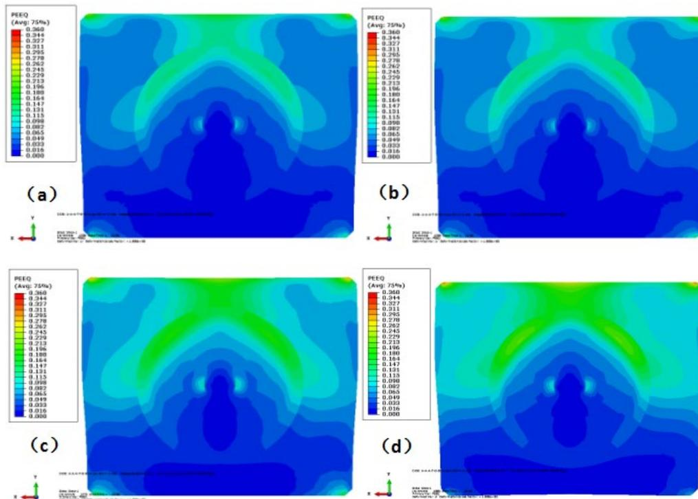
**Fig.4** - Equivalent strain of as-cast bloom under different reduction amount (centre solid fraction 0.55):
