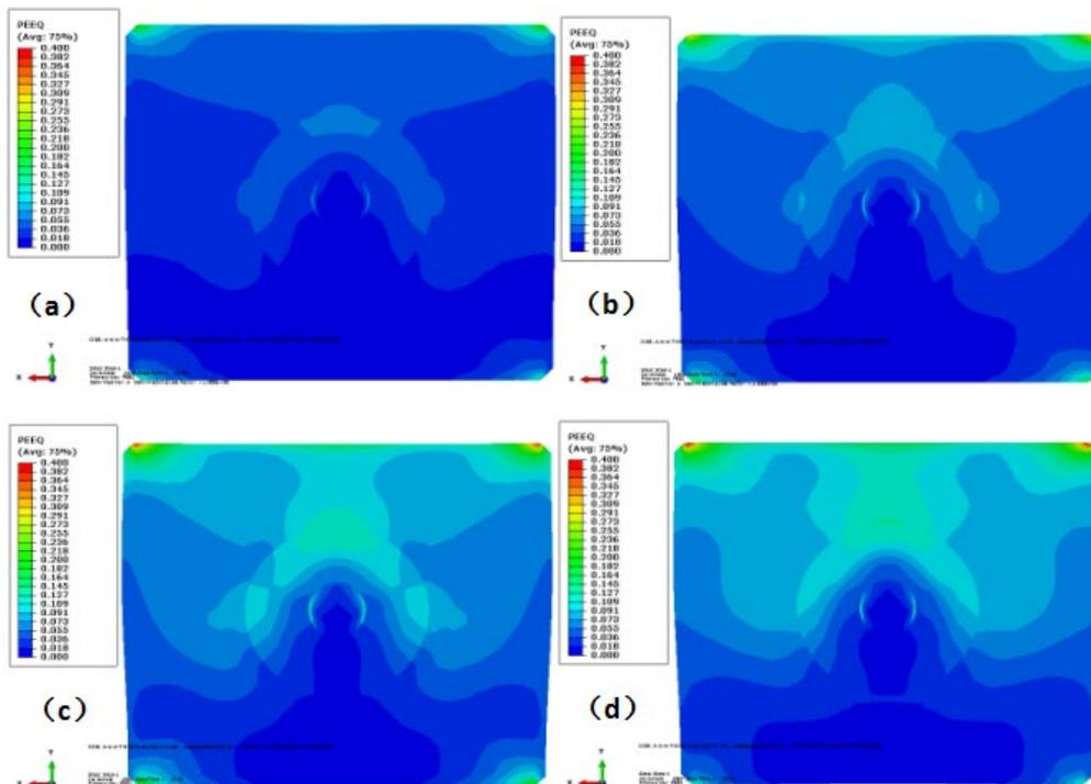
**Fig.5** - Equivalent strain of as-cast bloom under different reduction amount (centre solid fraction 0.66):
