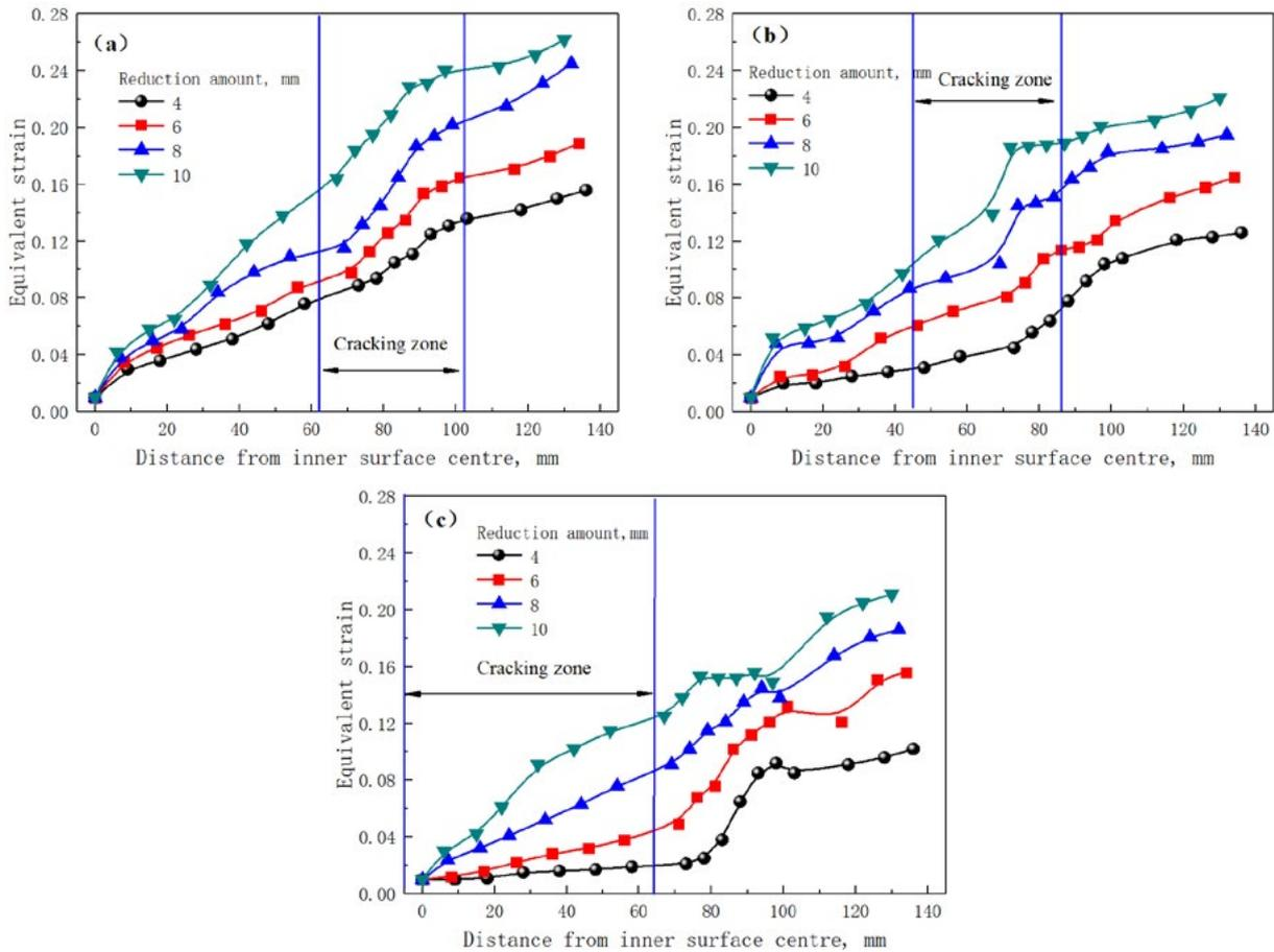
**Fig. 7** - Equivalent strain distribution for cracking zone in the inner transverse section of the bloom: (a) centre solid fraction 0.55; (b) centre solid fraction 0.66; (c) centre solid fraction 0.79.
