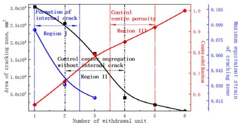
**Fig. 9** - Area of cracking zone, centre solid fraction and maximum equivalent strain in cracking zone under a number of withdrawal units.
