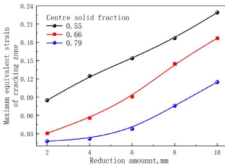
**Fig. 8** - Influence of reduction amount and reduction zone on the maximum equivalent strain of cracking zone.
