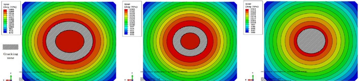
**Fig.2** - Temperature distribution and cracking zone under different reduction position.
