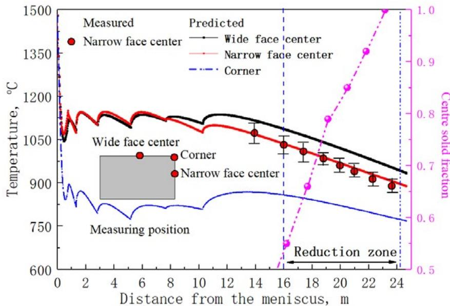
**Fig.3** - Comparison between the calculated and the measured temperature of the bloom narrow surface center.
