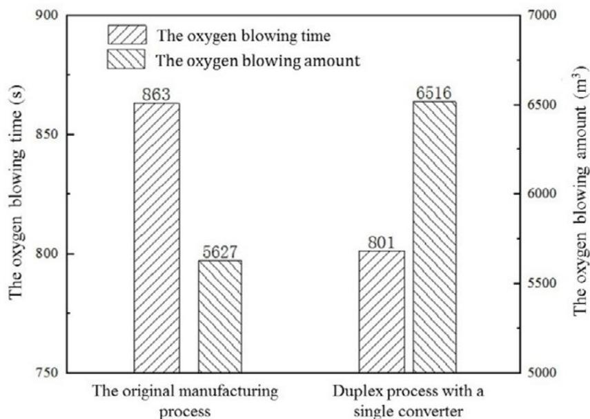
Fig.2 - Comparison of the oxygen blowing time and amount in different manufacturing processes.
