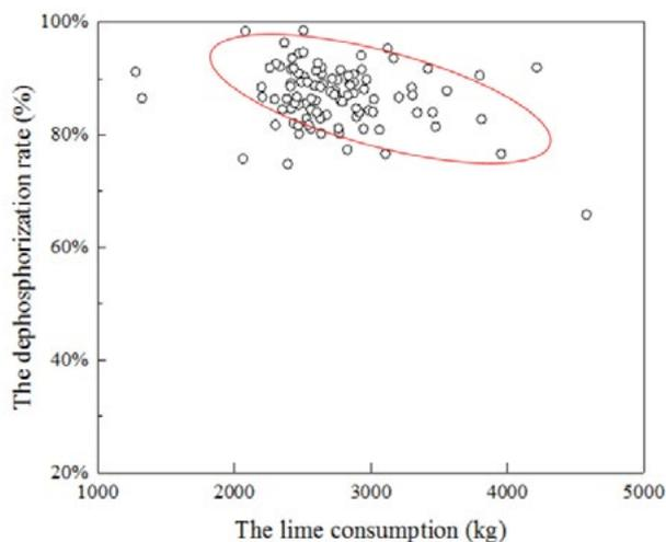
**Fig.4** - Scatter plot of lime consumption and dephosphorization rate.
