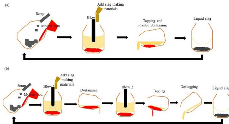
**Fig.1** - Duplex process with a single converter (a) the original process flow chart of a factory (b) the process flow chart of a factory using a single converter double method.
