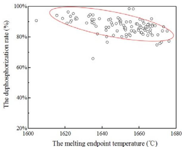
**Fig.3** - Scatter plot of melting endpoint temperature and dephosphorization rate.
