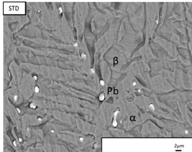
**Fig.7** - SEM micrograph of standard leaded brass faucet microstructure with phase distribution and Pb after casting process.
