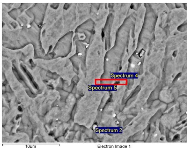
**Fig.12** - SEM micrograph of N3 composition with EDX analysis points.
