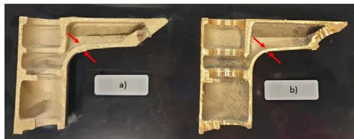
**Fig.14** - Cross-sectional area of a) standard, b) N3 brass samples after casting.
