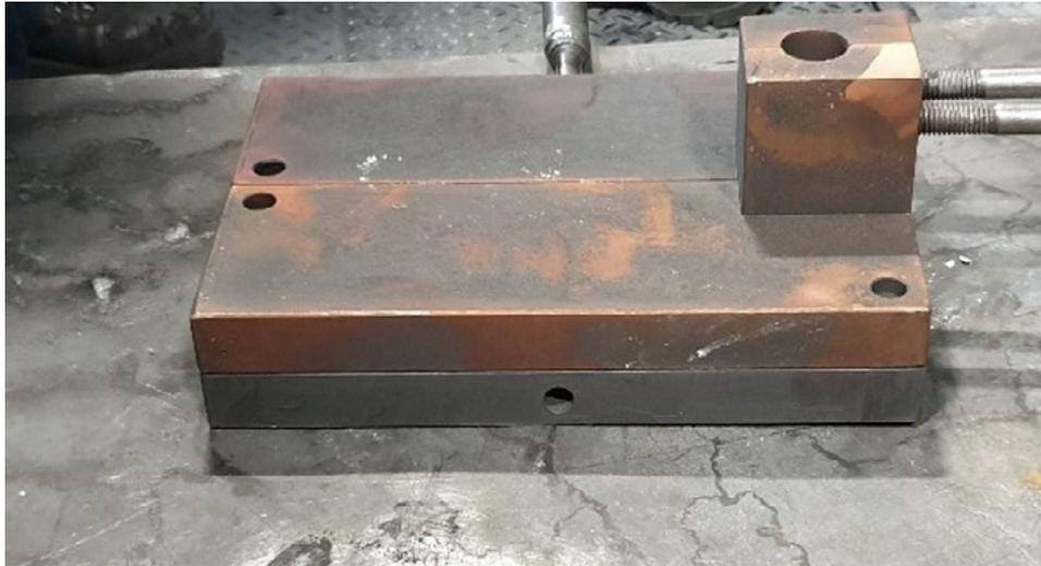
**Fig.2** - Strip fluidity test mould.
