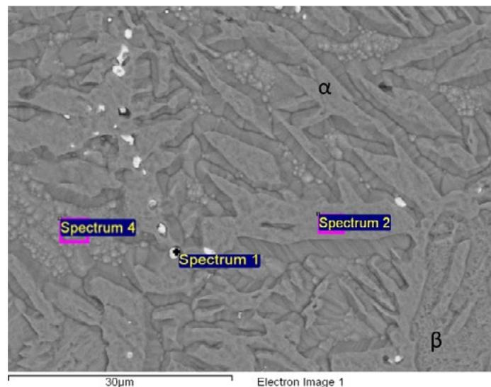
**Fig.10** - SEM micrograph of the brass faucet with A3 composition.
