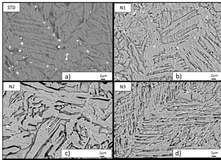
**Fig.11** - Comparison of microstructural images of (a) standard (b) 0.0055 wt.% (c) 0.03 wt.% (d) 0.05 wt% nickel-added cast compositions.
