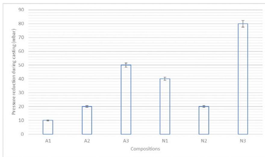
Fig.4 - Filling pressure change during casting of the composition.
