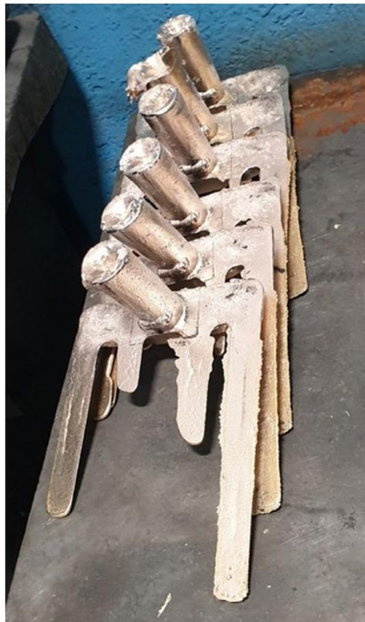
**Fig.3** - Photographic view of strip fluidity test.
