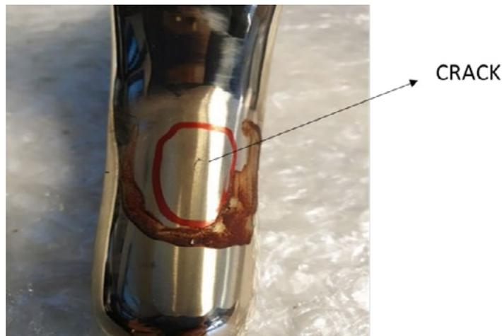
**Fig.13** - Crack sample of the faucet surface.
