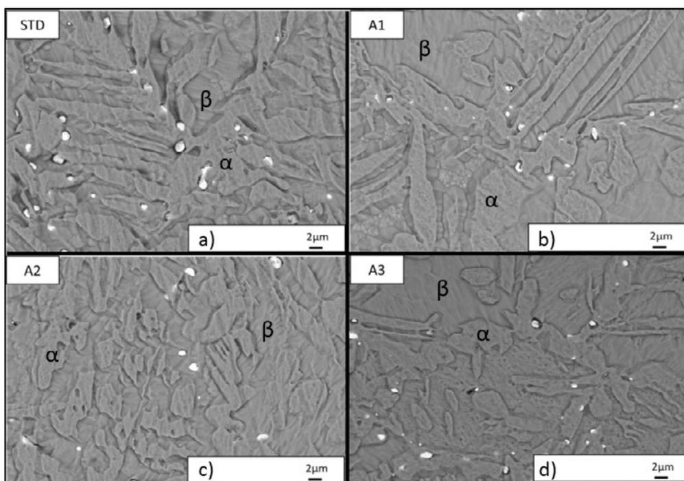
**Fig.8** - Comparison of the microstructure images of the standard leaded brass composition with (a) standard (b) 0.0055 wt% (c) 0.03 wt.% (d) 0.05 wt.% aluminum added compositions
