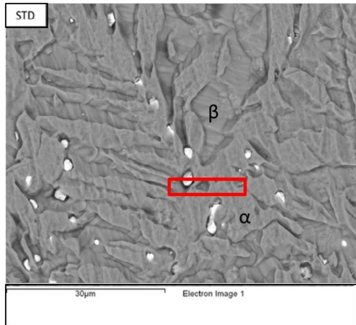
**Fig.9** - SEM micrograph of the faucet with standard leaded brass composition.
