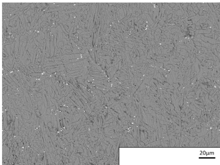
**Fig.6** - SEM image of the standard leaded brass faucet after casting process.
