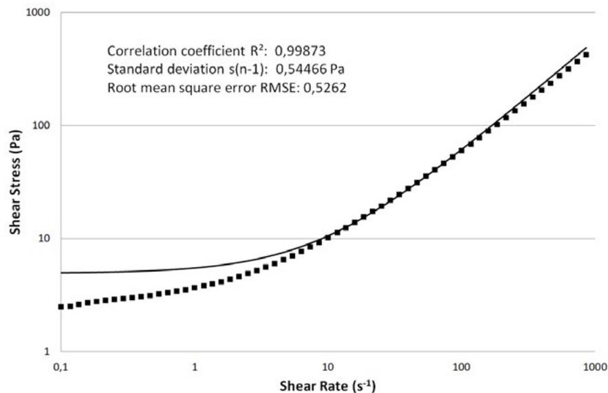
**Fig.4** - Bingham fitting of liquid casting powder sample.
