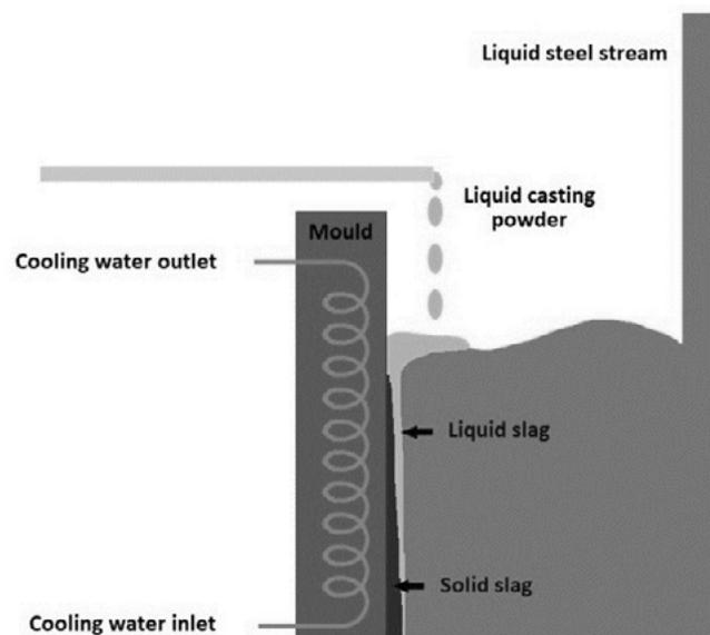
Fig.6 - scheme of liquid powder functioning in mold.
