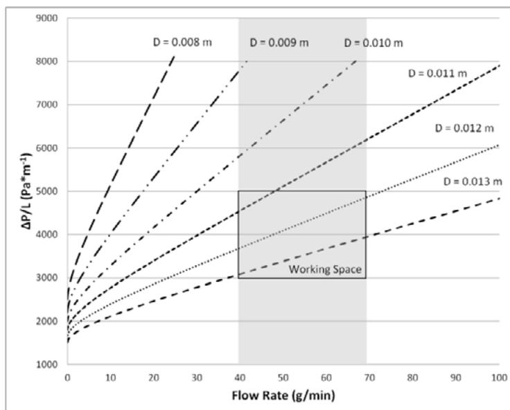
**Fig.5** - Definition of actual working space for real application of a liquid casting powder.
