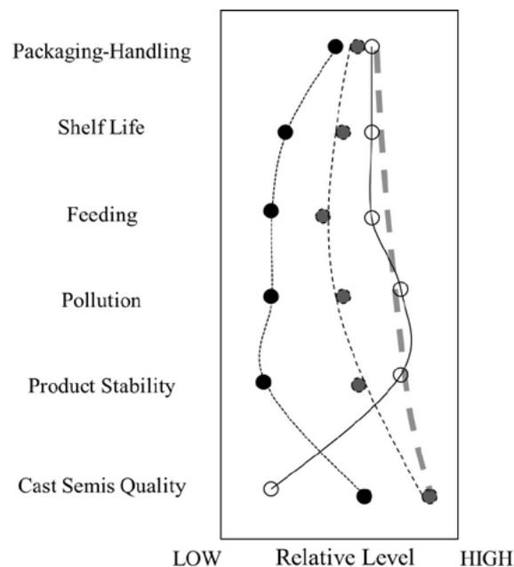
**Fig.1** - Elements of perceived quality for loose powder mold flux (black dots), granular mold flux (grey dots) and oil for continuous casting (white dots).
