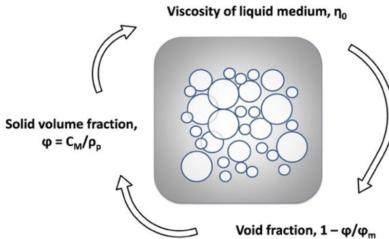
**Fig.2** - Elements describing solid-liquid dispersion system.
