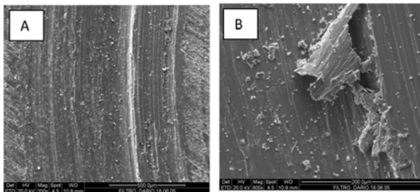
**Fig.16** - SEM-SE and SEM-BSE micrographs of CuSn12 bronze with DLC coating. A. SEM-SE micrograph. B. SEM-BSE micrograph. C. SEM-BSE micrograph at high magnification
