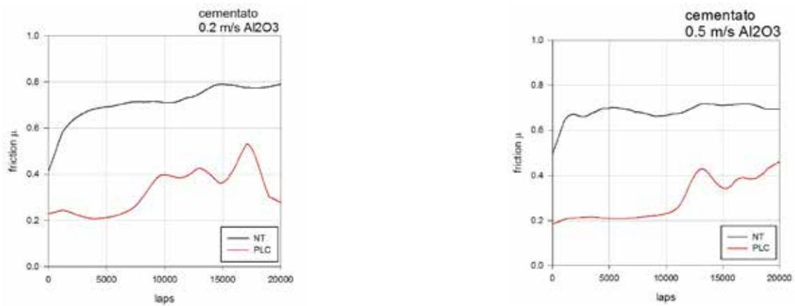
**Fig.11** - Friction behavior during sliding for CuSn12 bronze as received (NT) and with DLC coating (DLC)
