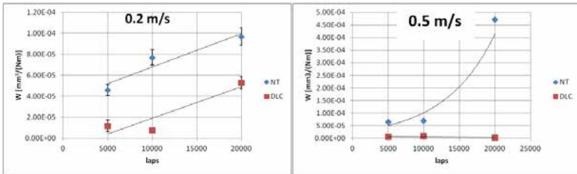
**Fig.13** - Wear rate graph of 16NiCrMo7 steel
