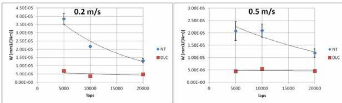
**Fig.14** - Wear rate graph of 41CrAlMo7 steel
