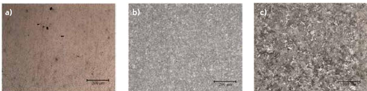
For all the metal alloys disc-shaped samples were cut from a 40 mm in diameter bar and then hardened with different treatment and coatings. Before the thin coating deposition, the substrate was carefully polished (Ra maximum 0.2) and
