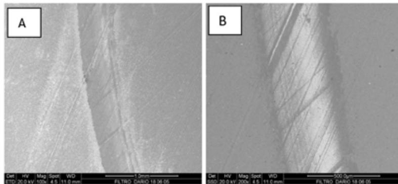
**Fig.19** - SEM-SE micrograph of wear track of 41CrAlMo7 untreated steel (A) and "duplex" treated (B)
