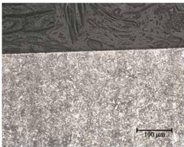
**Fig.3** - SEM-BSE Micrograph of 41CrAlMo7 with "duplex" treatment
