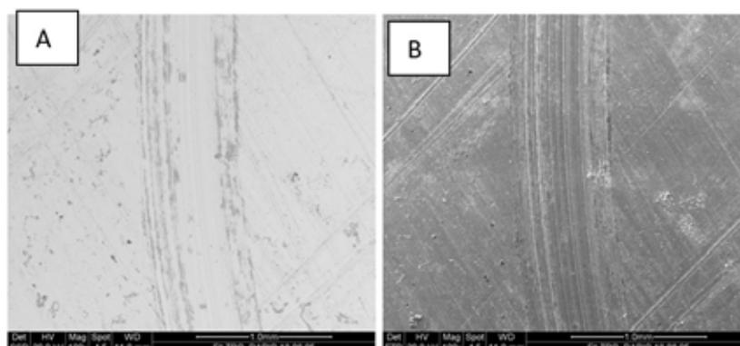
**Fig.18** - SEM-SE (A) and SEM-BSE (B) micrographs of 16NiCrMo7 steel with PLC coating
