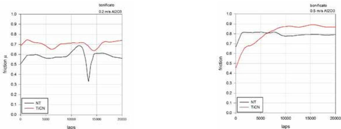
**Fig.10** - Friction behavior during sliding for 16NiCrMo7 carburized (NT) and with PLC coating (PLC)
