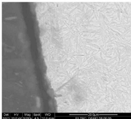
**Fig.6** - SEM-BSE Micrograph of bronze with DLC coating
