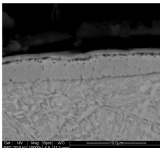
**Fig.4** - Optical Micrograph of carburized 16NiCrMo7 with PLC coating
