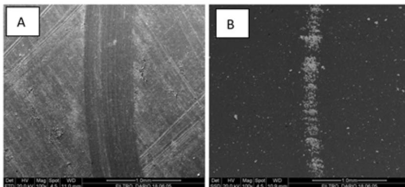
**Fig.20** - wear rate comparison of the solutions analyzed
