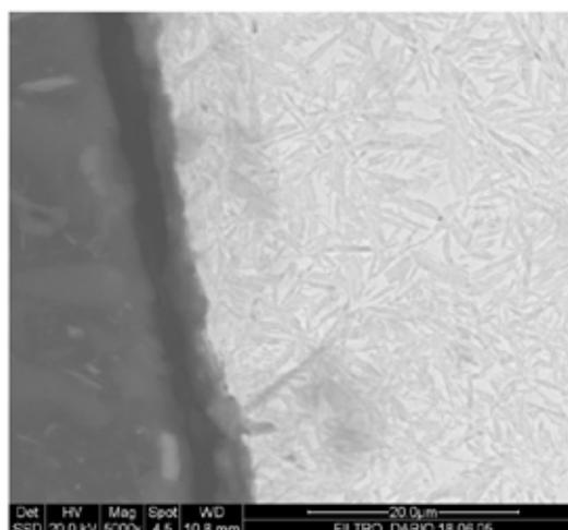
**Fig.5** - SEM-BSE Micrograph of carburized 16NiCrMo7 with PLC coating
